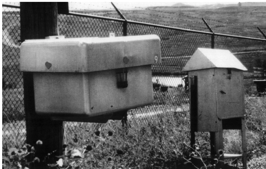
Figure III-56. Air samplers used by the Rocky Flats Plant (left) and the Colorado Department of Health (right) in the mid-1970s and beyond. EG&G Rocky Flats photo number 28761-6 dated ~1980. A schematic of the insides of these samplers is included later in this chapter.
