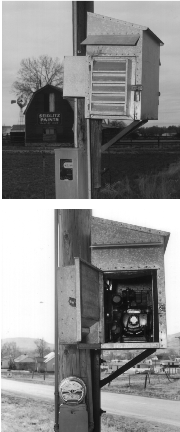
Figure III-54. Low-volume community air sampler maintained by the Rocky Flats contractor in the 1950s. In the upper photo, the sampler housing is closed, illustrating louvered door through which air enters. In the lower photo, the sampler housing is open, illustrating air filter and pump assembly. EG&G Rocky Flats photo numbers 01619-00 dated May 9, 1956, and 02196-00, dated March 20, 1957.
