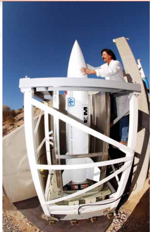
An electromagnetic missile launcher being prepared for a 2005 test launch at Sandia
