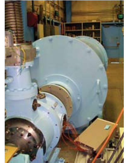
A series of gas gun projectile experiments at Sandia's STAR facility complemented experiments at the Z machine. The gun experiments subjected water samples to multiple shocks at increasing pressures.
