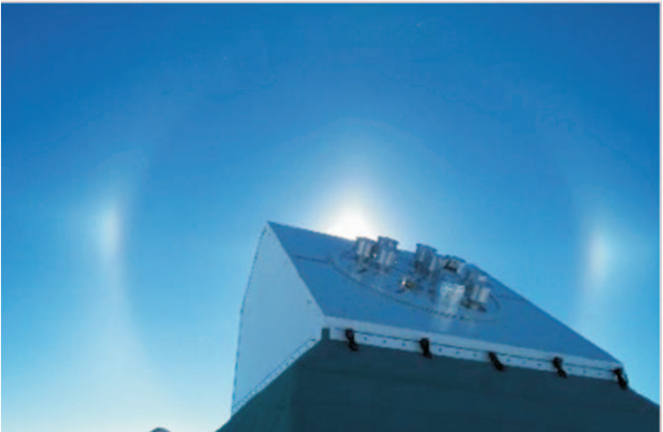
DASI is a 13-element interferometer designed to measure temperature and polarization anisotropy of the Cosmic Microwave Background (CMB) Radiation over a large range of scales with high sensitivity. The instrument operates from the NSF Amundsen-Scott South Pole station. Funding for DASI comes from the NSF Office of Polar Programs. The Center for Cosmological Physics (CfCP) provides additional support at the University of Chicago. (Photo Credit – John Yamasaki and the DASI Collaboration, 2002)
