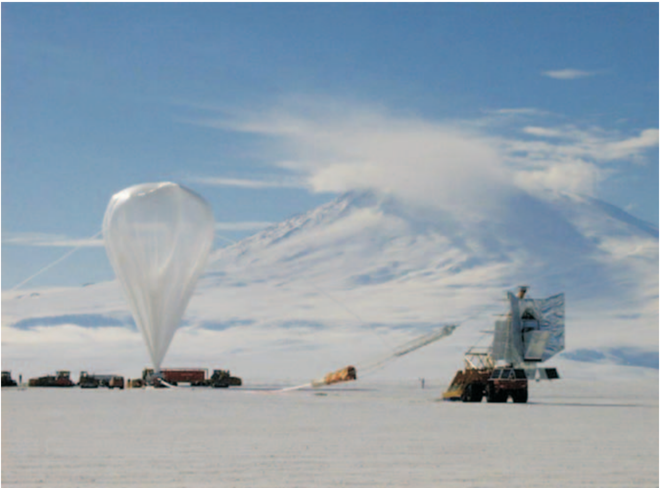
With Mt. Erebus as a backdrop, personnel inflate the 1 million m 3 (28 million cubic foot) balloon which will carry the BOOMERANG telescope on its 10 day trip around the Antarctic continent. In order to make its exquisitely sensitive measurements, BOOMERANG was lifted above 99% of the atmosphere to an altitude of 35km (120,000 ft). Primary support for the BOOMERANG project came from NSF and NASA in the United States; the Italian Space Agency, Italian Antarctic Research Programme and the University of Rome La Sapienza in Italy; and the Particle Physics and Astronomy Research Council in the United Kingdom. The Department of Energy's National Energy Research Scientific Computing Center provided supercomputing support in the United States. (Photo credit – Phil Mauskopf, University of Wales)
