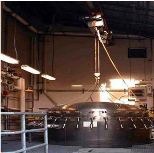
Figure 14. Alkaline Hydrolysis as a carcass disposal method can be made mobile, and destroys most FAD agents at the same time. However, capacity is limited and there are environmental health issues.
