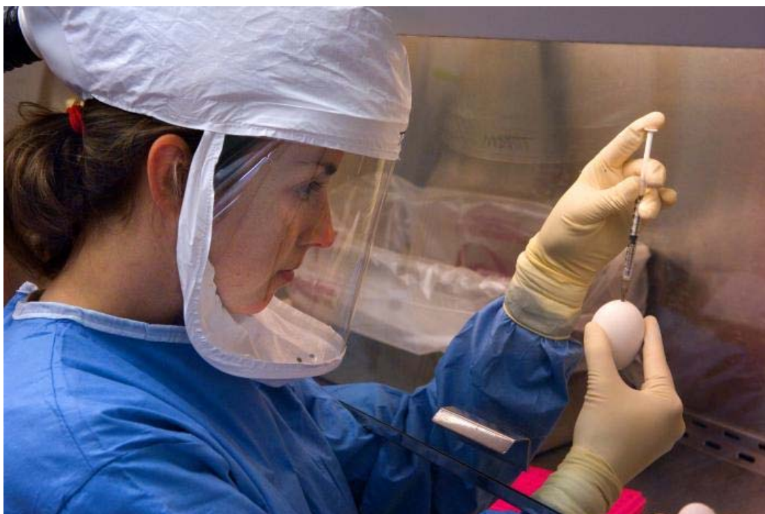
Figure 15. A microbiologist inoculates a 10-day old embryonated hen's eggs with a specimen containing an H5N1 avian influenza virus inside a biological safety cabinet (BSC) within the Biosafety Level 3-enhanced laboratory. This experiment was part of a study to investigate the pathogenicity and transmissibility of newly emerging H5N1 viruses. Airflow within the BSC prevents any airborne virus from escaping the confines of the cabinet.
