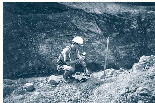
OSM geologist Robert Welsh uses Global Positioning System to locate a mine survey control point in relation to active mining operations in the State of Washington (photo by OSM).
