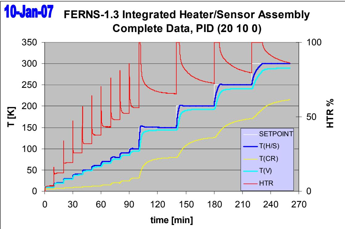
While T(H/S) gives the best control, the sensor T(V) gives a better indication of sample temperature (see below). But using T(V) as the control sensor gives much poorer
