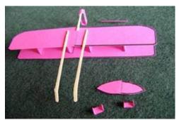
While the glider is upside down –smear glue on the tail support, hang the tail assembly on the tail support.
