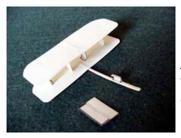
A 7/8" block from the large end of a toothpick for weight glued to the top of your toothpick airframe should provide balance. Place it as far forward as possible. Prepare your glider to fly using the "tuning" instructions on the next page.
