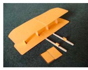
After the wing assembly is dry, glue the elevator in place carefully. Two 5/8" long blocks of toothpick from the wider, heavier end of a toothpick should provide enough balance weight. Consult "Final Tuning For Wright Biplanes" on page 10.
