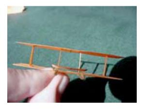
The TA Wright '01 as it appears in the "head on" view for tuning. This glider's wings are warped in opposite directions. The wing on the right is warped up, while the left hand wing is warped down. Twist the wings gently, in steps to equalize the lift on both sides. Most Wright flyers need some "up" elevator, as shown above. The tuning instructions on this page apply to all Toothpick Airforce aircraft.
