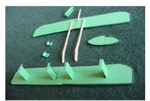
See page 8 for making strut "feet." The struts are positioned and glued in place, the strut feet bent to right angles from struts. The wings are upside down.
