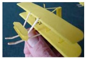
Grasp your toothpick flyer by one of the landing skids, and thrust it forward gently. Add "up" elevator by bending the leading edge of the elevator up and back.
