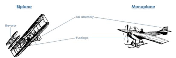
Biplanes have two wings with struts between for strength and support. The Wright elevator was in front.
