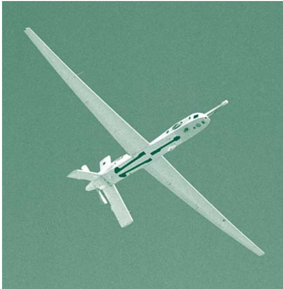
Above: The Altus II uninhabited aerial vehicle, built by General Atomics Aeronautical Systems, Inc., was chosen for its slow flight speed of 70 to 100 knots (80 to 115 mph), long endurance, and high-altitude capability (up to 65,000 feet). (Image courtesy of NASA/Dryden/Tom Tschida)
