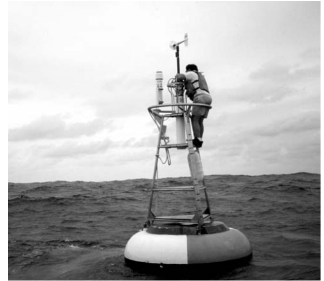
Above: A worker maintains a Tropical Atmosphere Ocean (TAO) buoy on the equatorial El Niño array in the Pacific Ocean. Developed under the auspices of the Tropical Ocean Global Atmosphere (TOGA) Program, these buoys measure ocean temperature at varying depths and give forewarning of El Niño or La Niña events. Although they offer limited coverage, the buoys provide a valuable ongoing record of ocean changes in conjunction with TOPEX/Poseidon and Jason-1 observations. (Image courtesy of the NOAA Photo Library)
