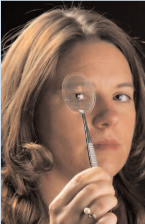
Christine Mitchell looks through a substrate that was made for the new cantilever epitaxy growth process, which gives potential for longer-lived and better-performing light-emitting diodes (LEDs).
