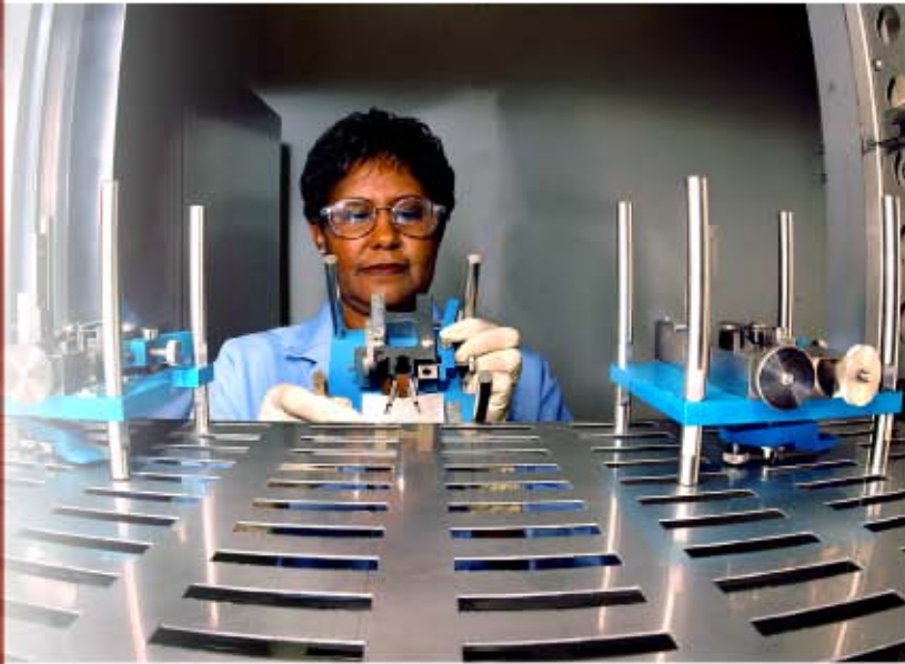
Annie Nickerson places power supply fixtures for neutron generators into a drying oven at Sandia's neutron generator production facility.
