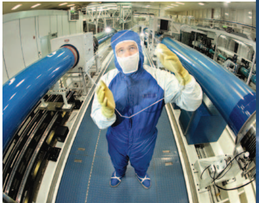
Technologist Benjamin Thurston examines the debris shield that protects the giant Z-Beamlet laser's focusing lens from flying debris when the Z accelerator fires.
