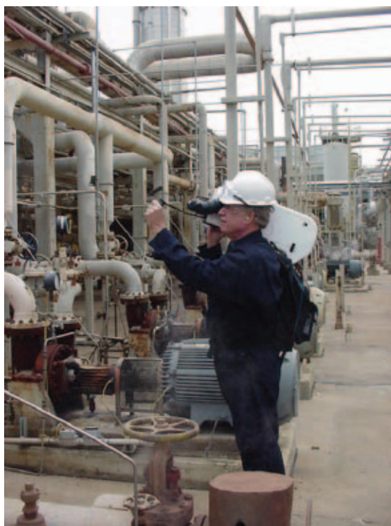
Sandia's portable gas-leak imager underwent major field tests in early 2003 at a Beaumont, Texas, refinery. Organizers from the American Petroleum Institute called the tests a major success. The imager is a backscatter absorption gas imaging system.
