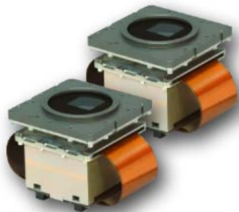
This Sandia satellite-based optical sensor package, only 1.5 cubic inches, provides a revolutionary level of processing. Sensing and signal processing are done at the equivalent speed of more than a gigabit per second, a level never before approached in a package this small.
