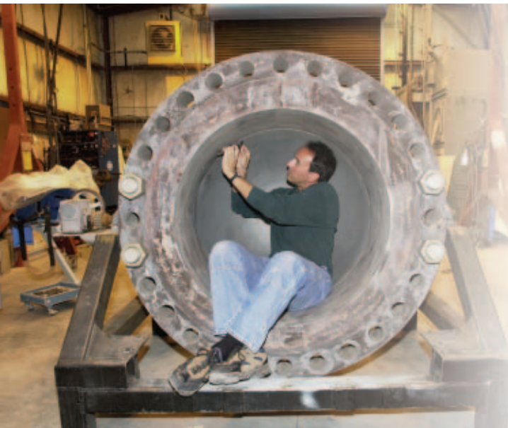
Richard Simpson of Sandia's Applied Nuclear Technologies department measures a weld in a 1/5-scale-model pressure vessel lower head assembly.
