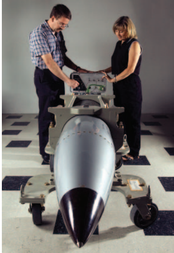
David Clements and Beth Connors test a B61-4 trainer using an aircraft monitor and control package that simulates the electronic control system of several types of military aircraft. These improved trainers have been distributed to military bases for use by flight-line ground crews in practice drills.
