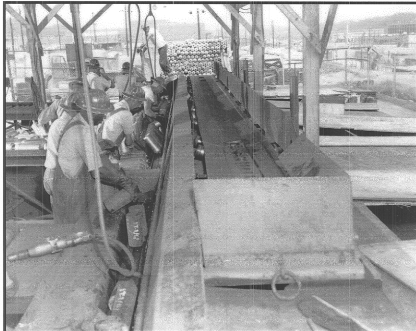
Photograph 4: Workers emptying flasks of mercury at the Y-12 mercury dumping shed. Pipelines carried mercury to the buildings that housed the Colex operations. (1955 photo ORO-55-762-3 courtesy of U.S. Department of Energy)
