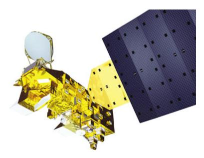
The Aqua satellite is the second flagship of NASA's Earth Observing System. Instruments aboard are designed to measure energy balance and temperatures in the land, sea, and atmosphere. (Image by Reto Stöckli)
