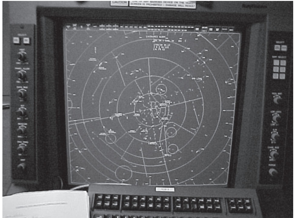
Figure 1: Standard Terminal Automation Replacement System Controller Workstation
