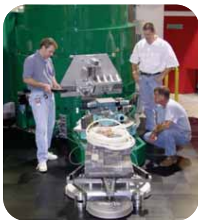
FIGURE 1. Engineer Colin Wrenn (right, standing) and machinist Mike Rinehart keep a watchful eye as engineer Mike Murbach (left) test drives the air-pad-supported under-carriage (loaded with lead bricks, in foreground) for the analyzer/detector section of the new thermal neutron triple-axis spectrometer at BT-7.
