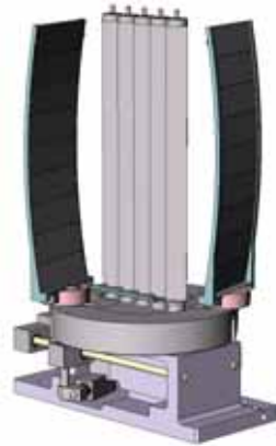
FIGURE 3. CAD image of the double crystal analyzer of which there will be 20 in the MACS detector system.
