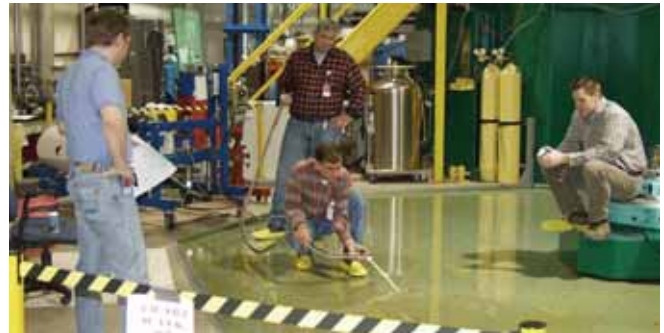
NCNR's Mike Murbach, Mike Gue, Mike Rinehart, and Colin Wrenn install the "dance floor" for the analyzer of the new BT-7 triple-axis spectrometer.
