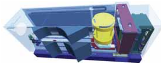
FIGURE 2. CAD image of the monochromating system for the MACS spectrometer. The "golden" doubly focusing monochromator was built and tested at The Johns Hopkins University.
