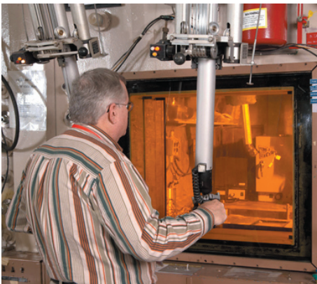
Years of experience with the manipulators enable the operators to perform tasks that require great dexterity.
