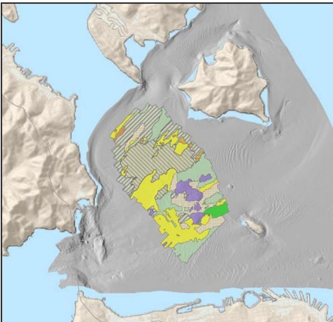
*The figure shows a side-scan habitat interpretation overlaid on a multi-beam survey near Angel Island. Approximately 120 km<sup>2</sup> of archived multibeam data and 50 km<sup>2</sup> of side-scan sonar data were interpreted for habitat characterization. Soft sediment was the dominant induration type and ranged from mud and sand to bimodal sediment of gravel, pebbles, and cobbles. Mixed and hard habitat types were relatively rare.*
