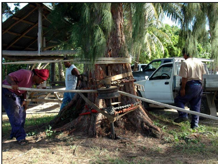
Pulley system for redirecting tow from truck to vessel
