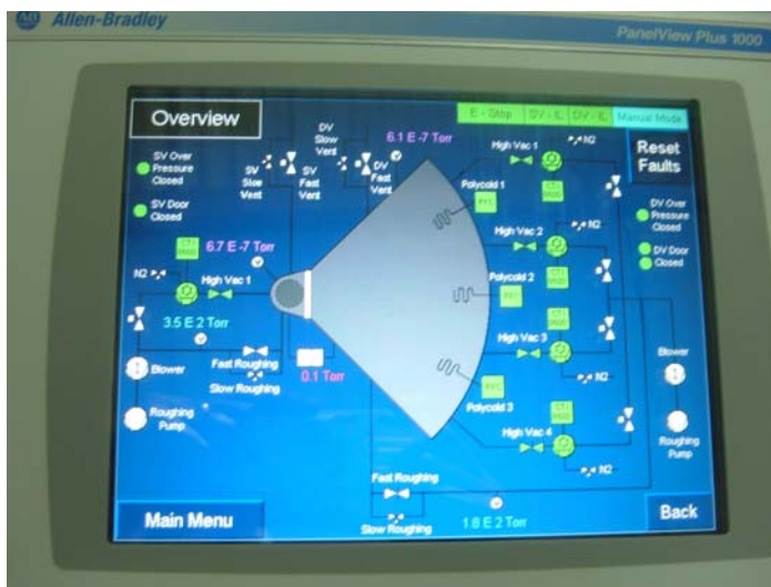
Final pump down values for the SEQUOIA sample and detector vessels
