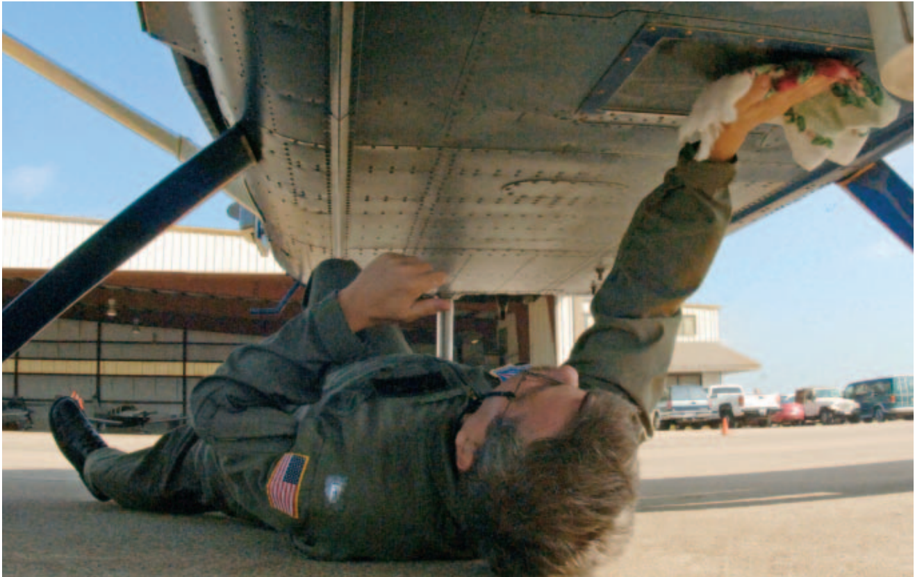
A member at CAP's West Houston Mission Base cleans the hyperspectral imaging window on a Gipsyland GA8 Airvan prior to an ARCHER mission that CAP performed for the U.S. Army Corps of Engineers.
