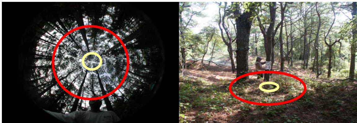
Figure 2. The larger the laser spot size, the greater the degree of target mixing. The two circles schematically illustrate the area illuminated by two laser pulses of differing diameters. Depicted on the left is an up-looking hemispherical view of tree canopy, whereas a ground-level view is shown on the right - both images taken on Assateague Island, MD.
