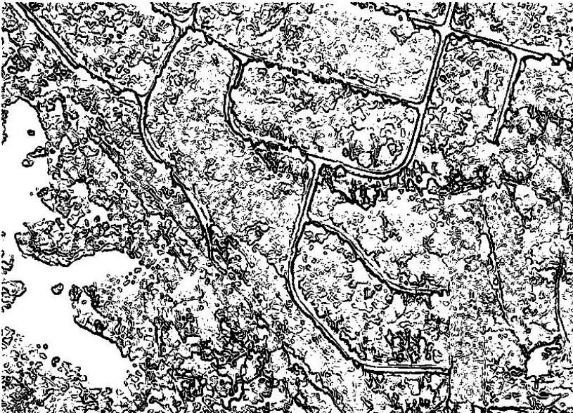
Figure 4. Sobel edge detector example.
