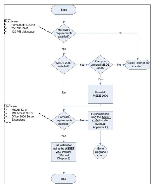
Figure G.1 - Full Installation Process
