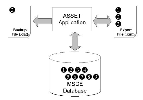
Figure 4.1 - Top-level ASSET Architecture
