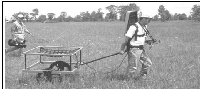
Figure 13. Typical EM Induction System
