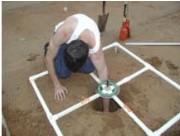
Figure K-2. Example of object leveling using object positioning template and integral leveling devices.
