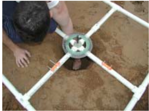
Figure K-2. Example of object leveling using object positioning template and integral leveling devices.
