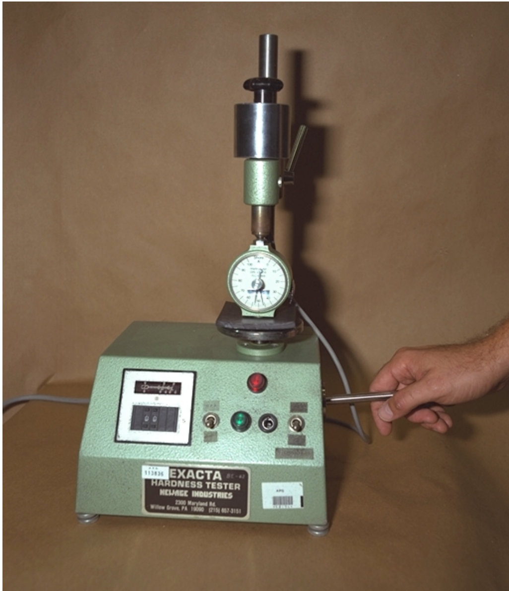
Figure 1. Durometer measurement of rubber specimen.
