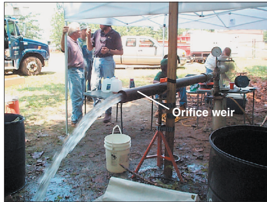
Pumping tests were conducted on six test wells during 2001, such as well 14FF55 above. The USGS used an orifice weir to measure pump discharge. The USGS collected chlorofluorocarbon samples from the wells and monitored water levels to better define aquifer hydraulic properties. Photo by Lester J. Williams, USGS.
