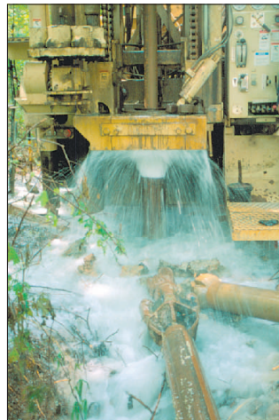
Pumping tests were conducted on six test wells during 2001, such as well 14FF55 above. The USGS used an orifice weir to measure pump discharge. The USGS collected chlorofluorocarbon samples from the wells and monitored water levels to better define aquifer hydraulic properties. Photo by Lester J. Williams, USGS.
