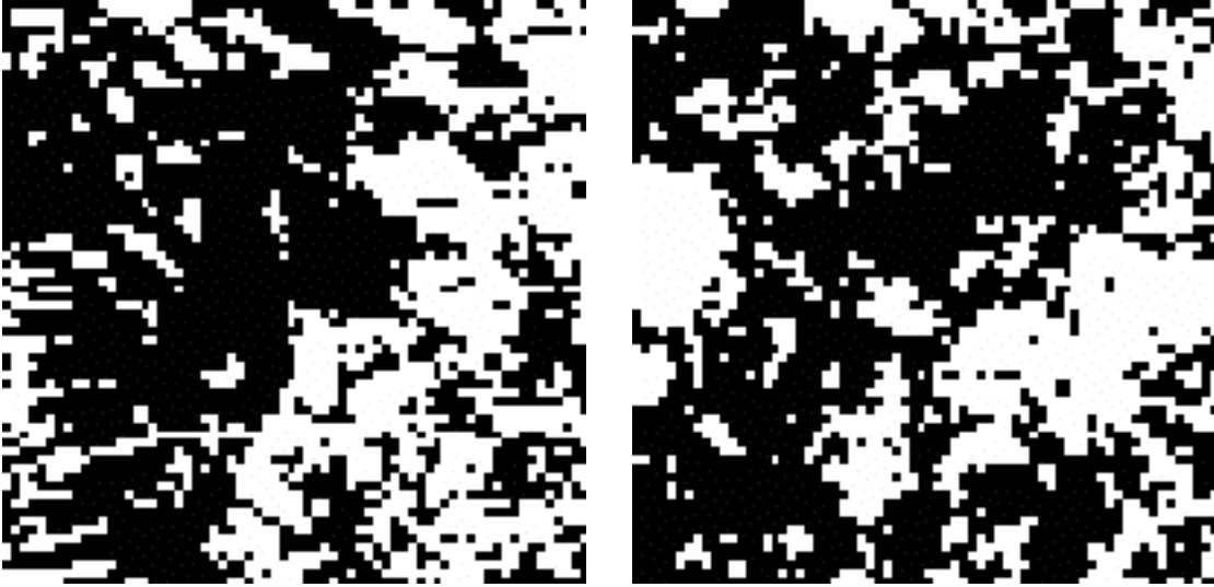
Figure 5. Indicator functions I(x,y) of a cloud field: white is cloud ( I=1 ) while black is a cloud-free area ( I=0 ). Cloud fraction A_c=0.4 . (Left) 68 km by 68 km MODIS image centered at ( 17.1^\circ S, 42.16^\circ W) acquired on August 9, 2001. (Right) a realization of a simulated field.
