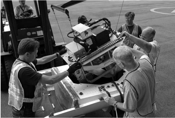
The ER-2 crew and AMPR team members reinstall the AMPR instrument in its hatch. (Clockwise from forklift: Kevin Kraft, Mike Kapitzke, Wayne Deats, Mark James, and Pat Lloyd).
