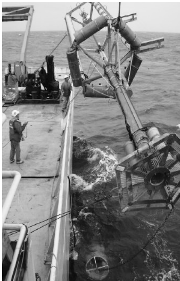
The ASIS being deployed off the back of the Ron Brown .
