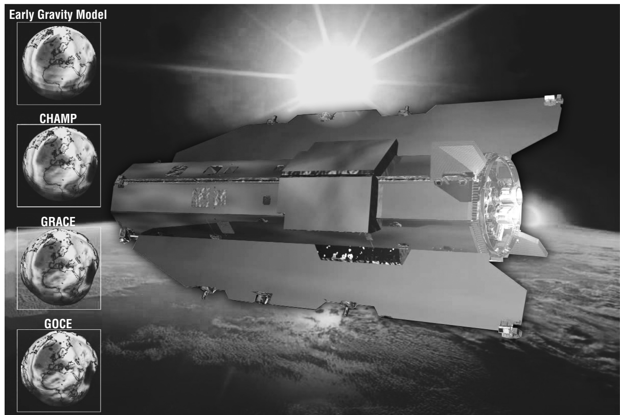
This is an artist's drawing of the European Space Agency's Gravity Field and Steady State Ocean Circulation Explorer (GOCE) Satellite, which is scheduled to launch in May 2008. GOCE will provide the most accurate measurements of the Earth's gravity field that have been obtained to date. GOCE improves on measurements from the Gravity Recovery and Climate Experiment (GRACE), Challenging Minisatellite Payload (CHAMP), and earlier Gravity Models. Credit: ESA/AOES Medialab.
