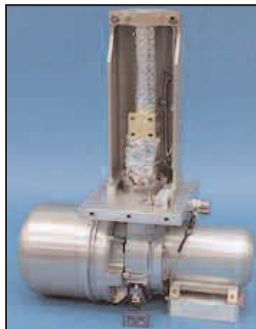
Figure 8. Northrop Grumman's high-efficiency cryocooler unit weighs less than 7 kilograms compared to previous state-of-the-art at 22 kilograms. Sixteen units have been ordered for various flight programs.
