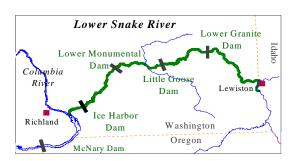
Over a period of 13 years (1962-1975), four dams were constructed on the lower Snake River. Ice Harbor, Lower Monumental, Little Goose, and Lower Granite dams are all run-of-the-river dams, meaning they pass water at about the same rate as it enters. They were constructed primarily for navigation and hydropower generation and provide almost no flood control. Also, lower Snake River water irrigates about 40,000 acres, mostly around the Ice Harbor pool.
