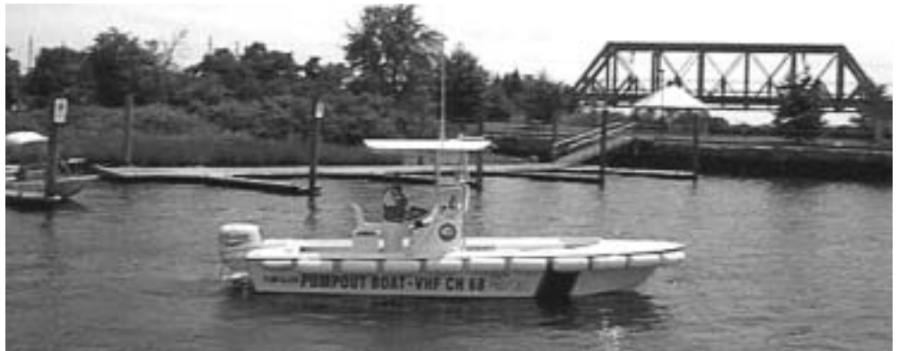
States have developed innovative techniques to provide services for recreational boaters through their Clean Vessel Act grant programs. A local Connecticut marina's sewage pumpout boat motors to a boat waiting to have its waste removed. Photo: Connecticut Department of Environmental Protection.
