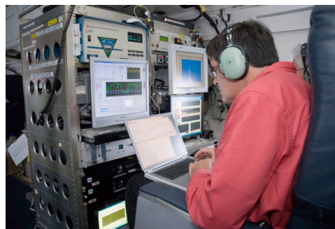
Dr. Jim Podolske of the Atmospheric Science Branch examines laser absorption spectrometer data of water vapor and carbon monoxide during a NAMMA science flight.
