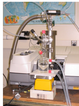
Multiphase reactor allows temperature-controlled studies of aqueous processes. The gases in equilibrium with solution are monitored with infrared spectroscopy.
