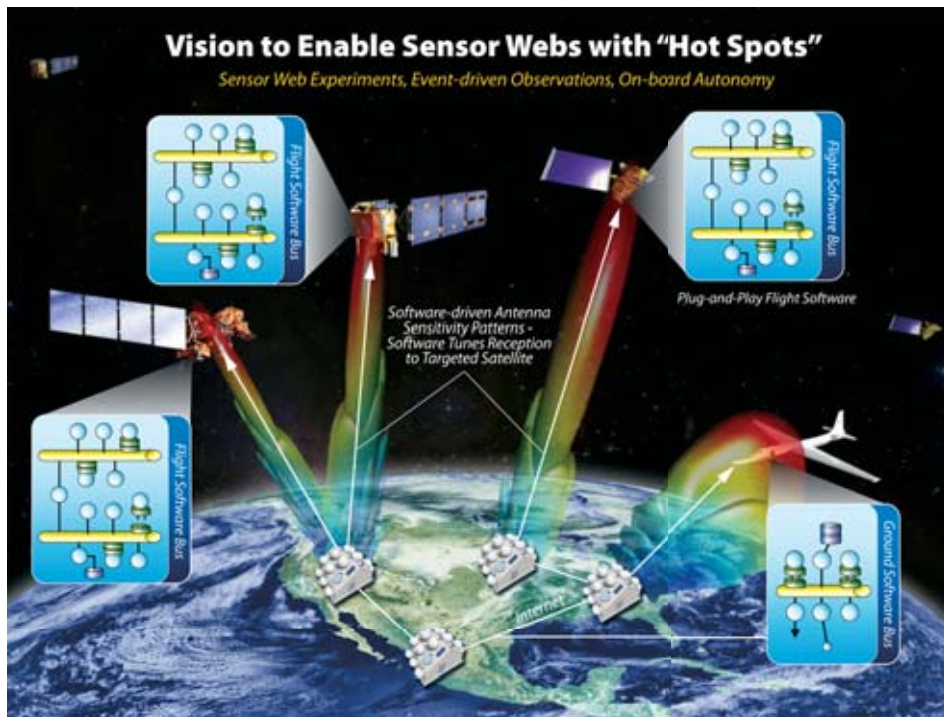
Figure 3. Sensor web vision with seamless communications between space and ground software elements.
