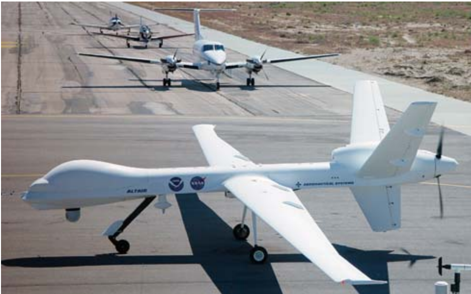
Figure 3. The Altair UAV developed for science missions (photo courtesy of NOAA).
