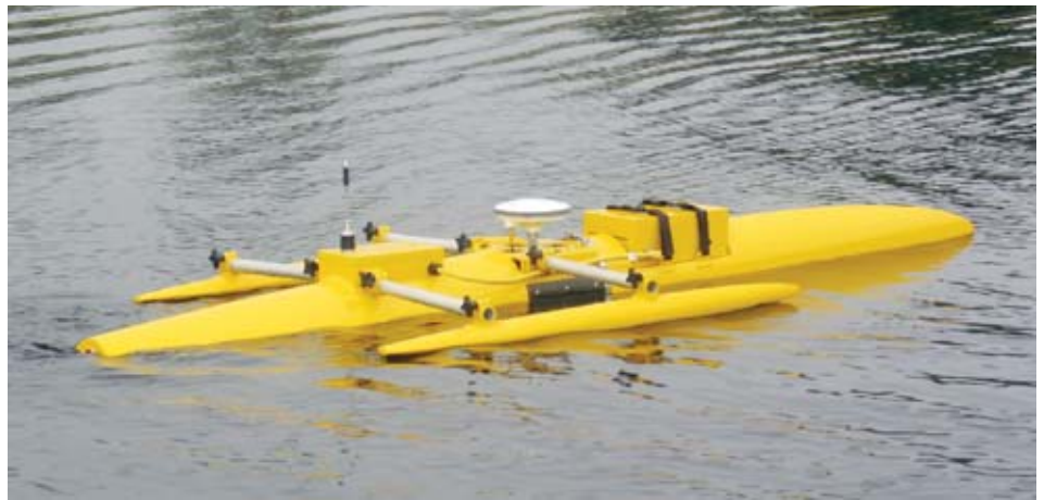
Figure 2. A USV designed for USGS (photo courtesy of Sea Robotics Corporation).
