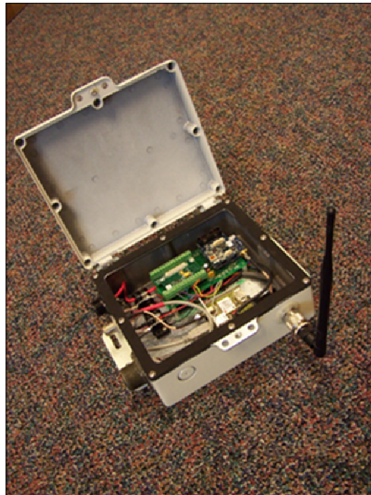
Figure 5. Prototype ground sensors developed by USGS
