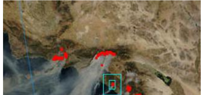
Figure 5: Active fire alerts for the recent October 2004 Southern California Fires. Red indicates active fires. The light blue box illustrates the background region used in the relative threshold detection.
