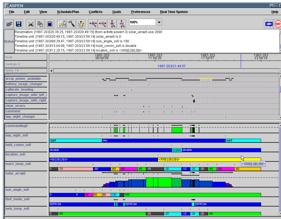
Figure 4: The ASPEN graphical user interface (GUI). The pull-down menus and buttons give options for modifying the plan. Activities are shown as black horizontal bars in the middle section. The values of resources and state variables over time are shown as colored blocks in the bottom section.
