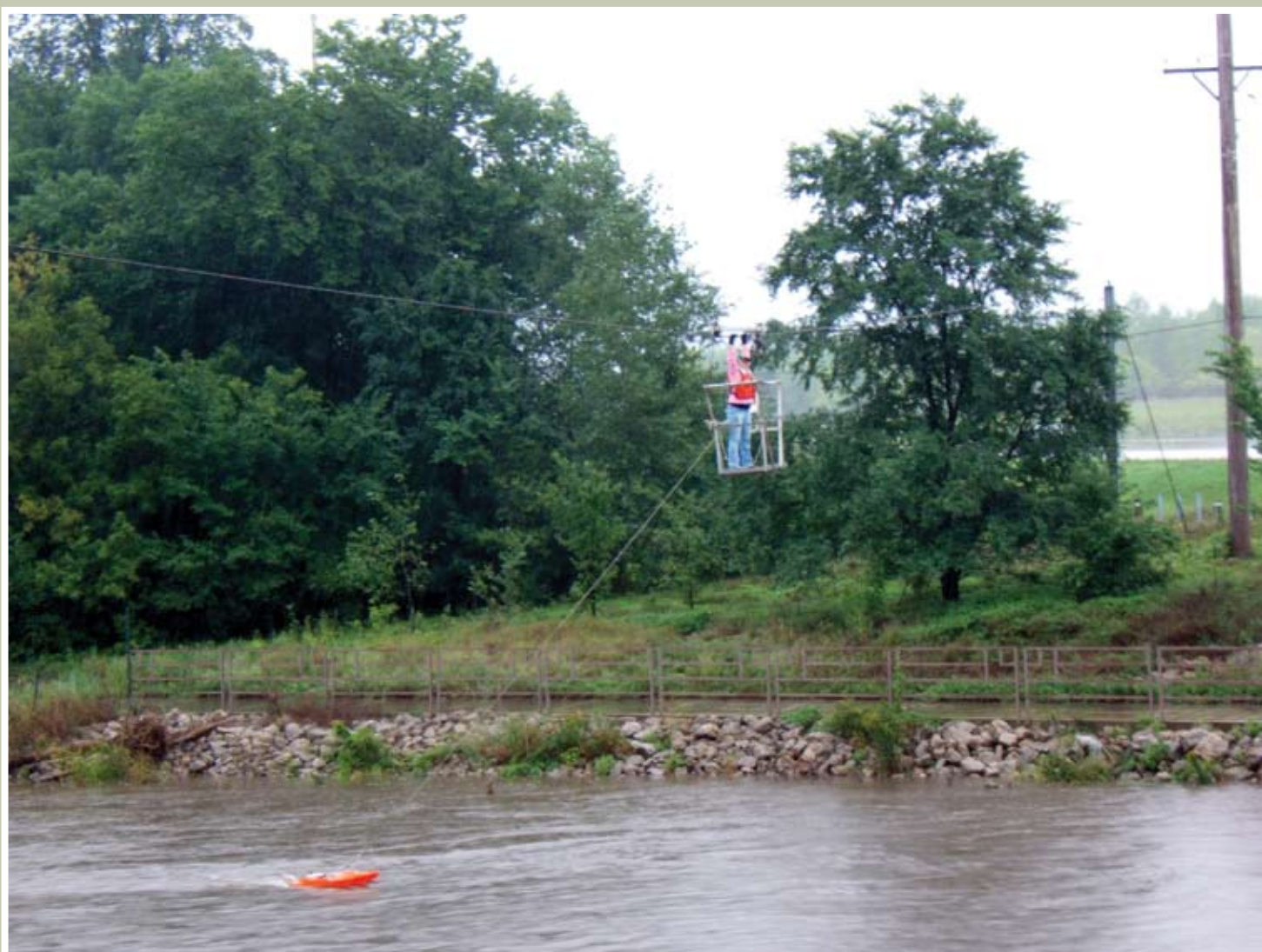
A cableway and acoustic Doppler current profiler measurement on the Zumbro River, Minnesota
