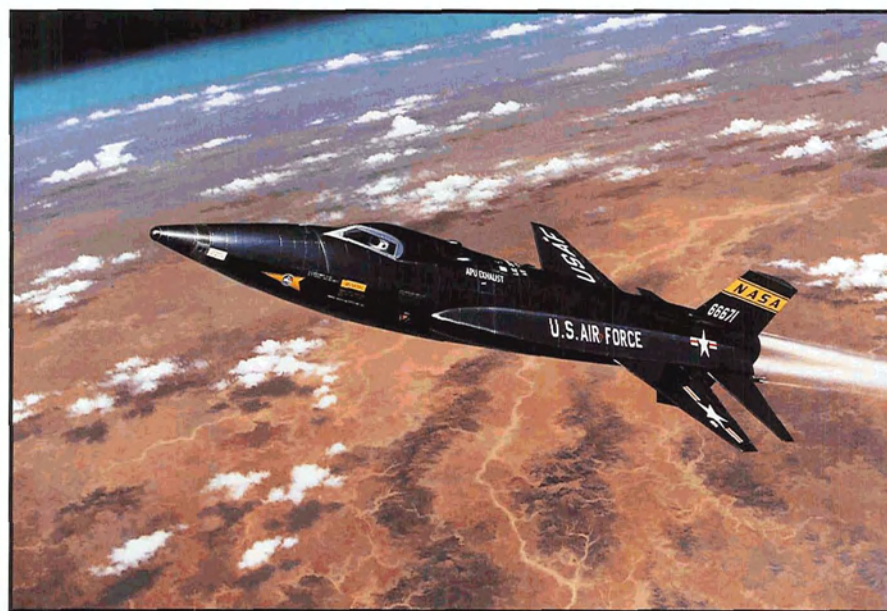
This painting by Stan Stokes of the X-15 rocket aircraft is part of the NASA Art Program. First flown in 1959 from the NASA High Speed Flight Station (renamed the NASA Flight Research Center that year and the Dryden Flight Research Center in 1976), the rocket-powered X-15 was developed to provide data on aerodynamics, structures, reentry characteristics, heating, reaction and other flight controls, instrumentation, and the physiological aspects of high speed, high altitude flight. Three were built by North American Aviation for NASA, the Navy and the Air Force. They made a total of 199 flights during a highly successful research program lasting almost ten years. Their speed and altitude records for winged aircraft remained unbroken until the Space Shuttle first returned from Earth orbit in 1981. (NASA Photo EC94 42909-1)
