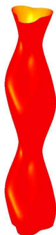
Figure 11. Capillary instability of a nanowire with an anisotropic surface energy with three-fold symmetry about the wire axis.
