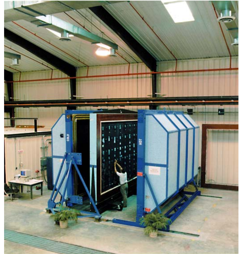
Rotatable guarded hot box in the Buildings Technology Center. The hot box is used to test the thermal performance of walls.
