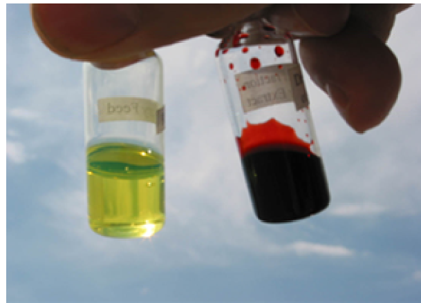
Examples of Hydrotreated Raffinate and Light Extract from Value Enhancement Process
