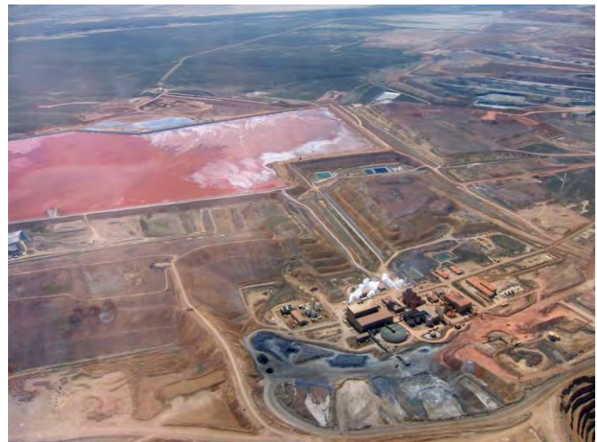
The Twin Creek Mine, Nevada, showing steam releases and consumptive water loss at the mill. The aqueous tailings dump, beyond, evaporates large amounts of water as well. It is likely red from the oxidation of waste minerals. Photo by Earthworks.
