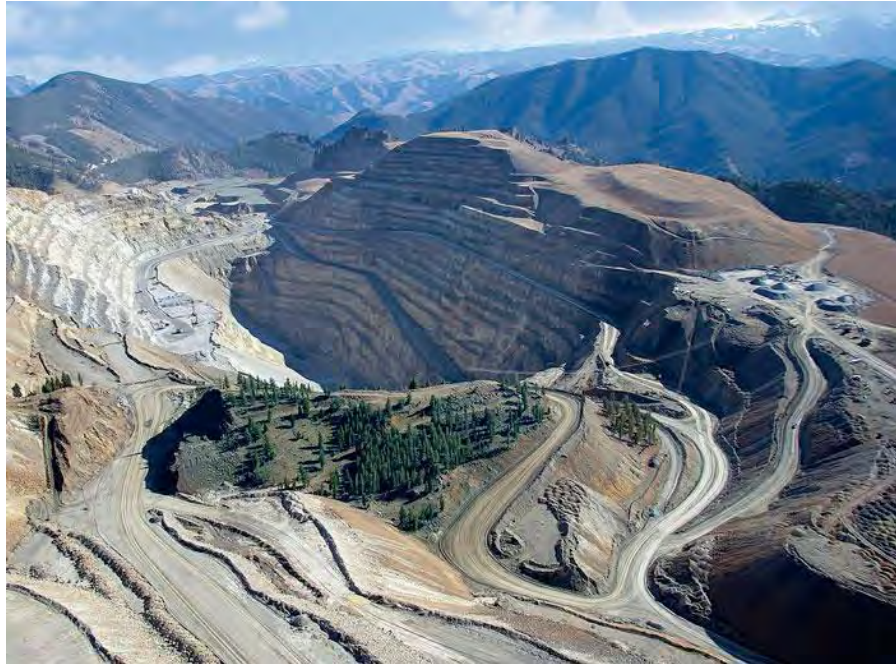
The Thompson Creek Mine in Idaho, an operation comparable in size to Hermosa. Although this mine processes more ore per day, the ultimate depth and width of the pit is similar: 1500 feet deep and 5,000 feet across ( source a ). Photo by Thompson Creek Metals.
