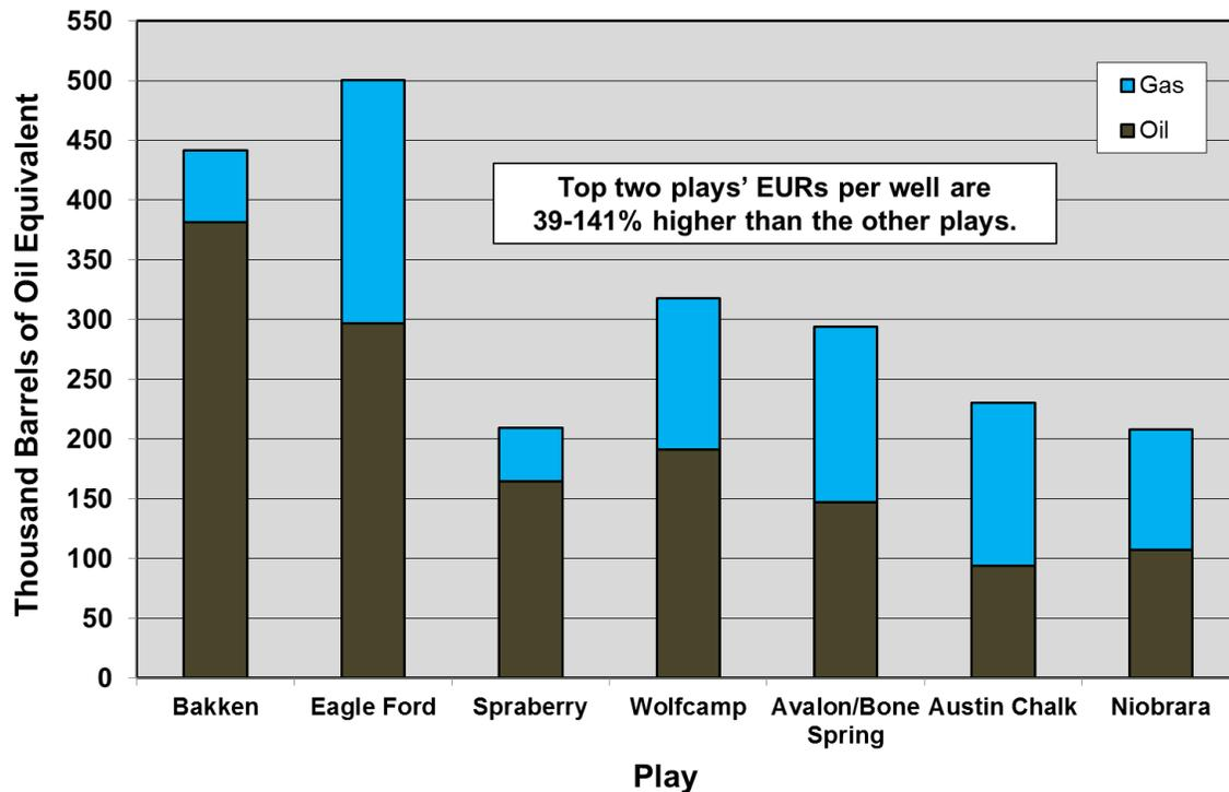
**Figure 2-94. Estimated ultimate recovery (EUR) of oil and gas per horizontal well of reviewed plays, on a “barrels of oil equivalent” basis.<sup>155</sup>**
