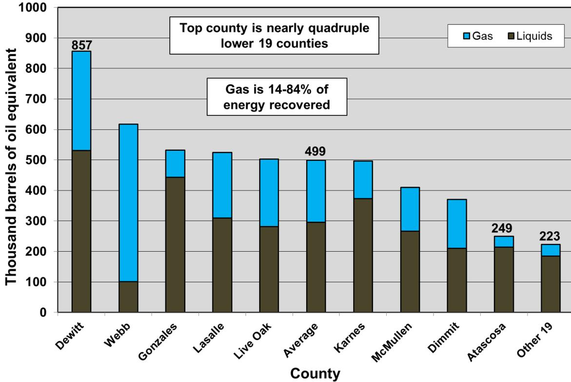
**Figure 2-47. Estimated ultimate recovery on a “barrels of oil equivalent” basis, including the energy value of gas, by county for the Eagle Ford play.<sup>76</sup>**
