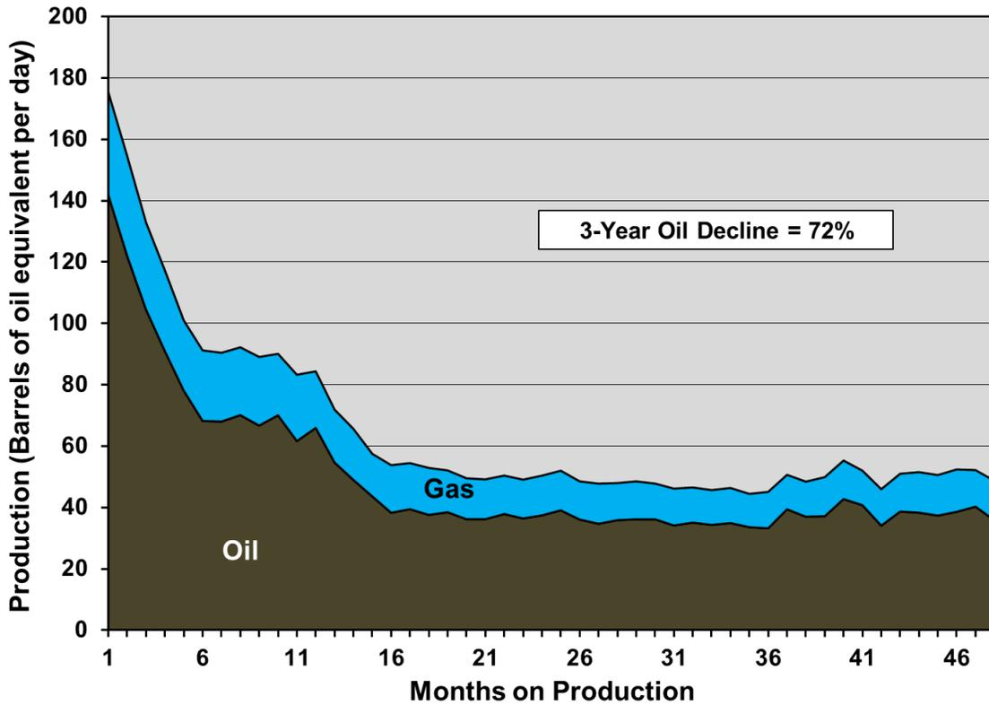
**Figure 2-61. Oil and gas average well decline profile for horizontal wells in the Spraberry play.<sup>96</sup>**
