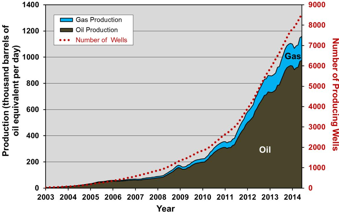
**Figure 2-11. Bakken play tight oil and gas production and number of producing wells, 2003 to 2014.<sup>23</sup>**
