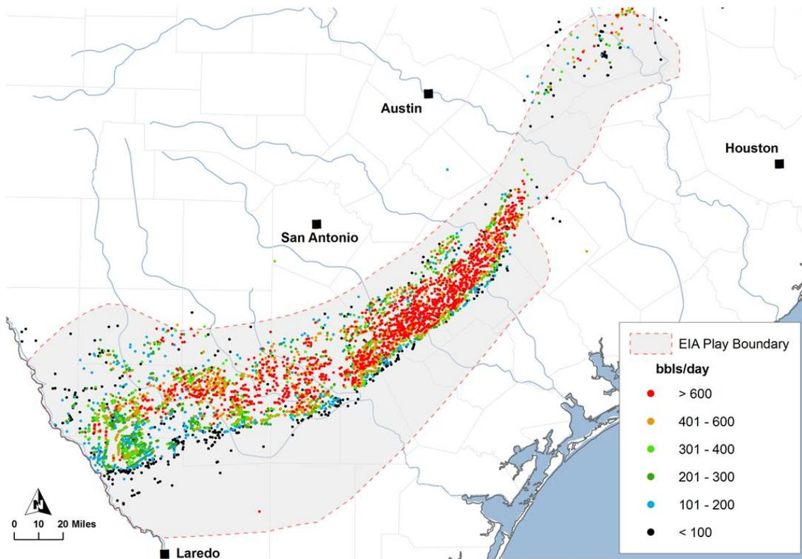
**Figure 2-28. Distribution of wells in the Eagle Ford as of mid-2014 illustrating highest one-month oil production (initial productivity, IP),<sup>53</sup> with EIA play boundary.<sup>54</sup>**
