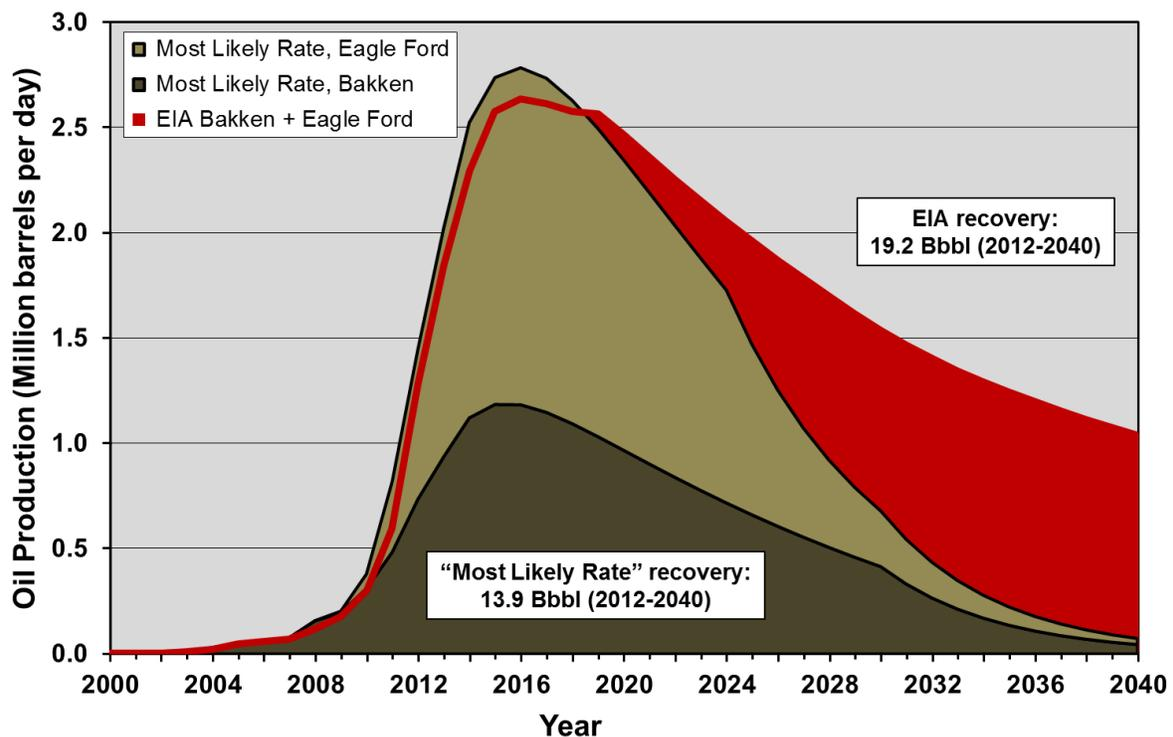
**Figure 2-95. “Most Likely Rate” scenarios (“Realistic” cases) of Bakken and Eagle Ford tight oil production compared to the EIA reference case, 2000 to 2040.<sup>157</sup>**
