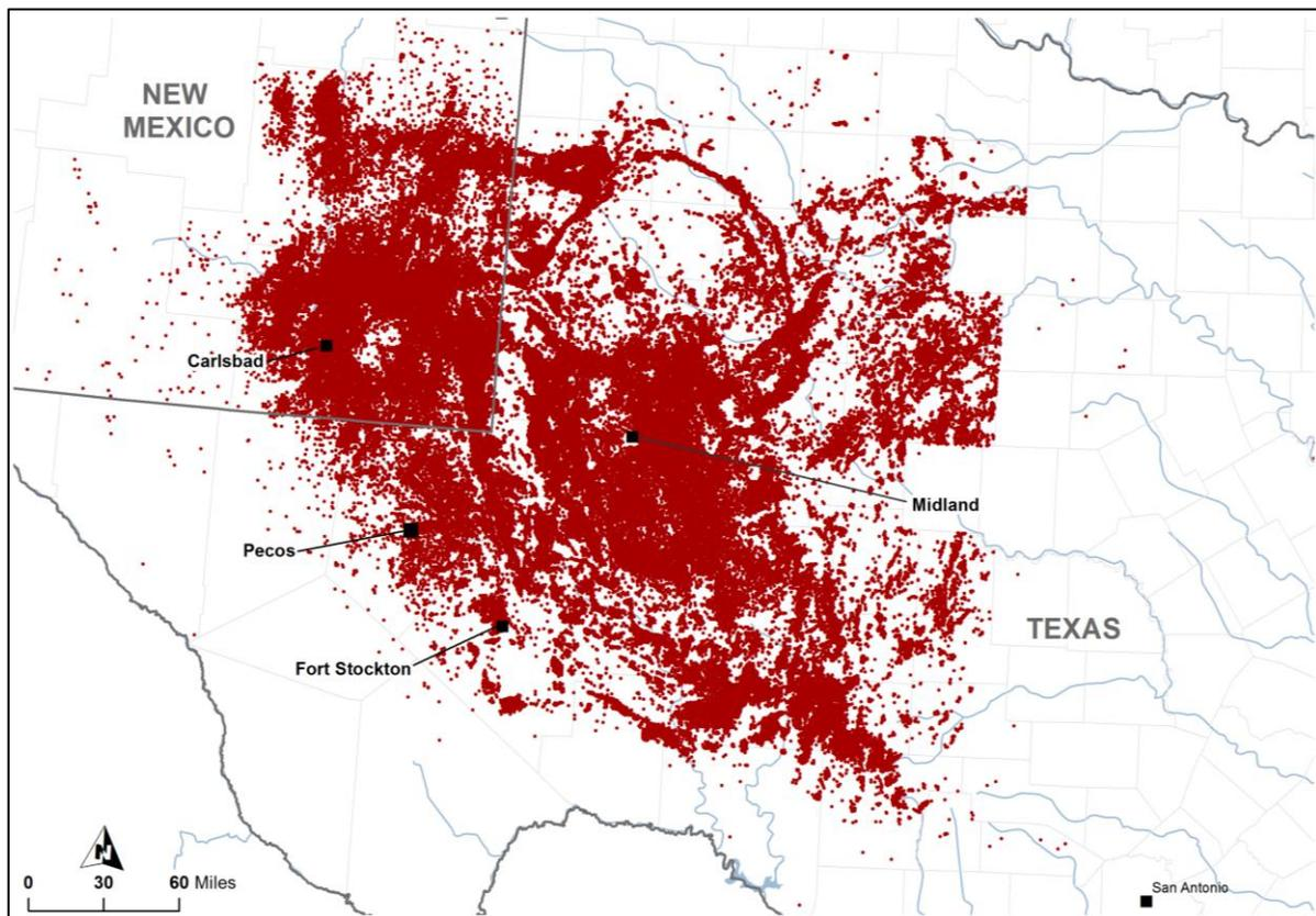
**Figure 2-54. Distribution of wells drilled since 1970 in the Permian Basin of Texas and southeastern New Mexico.<sup>89</sup>**
