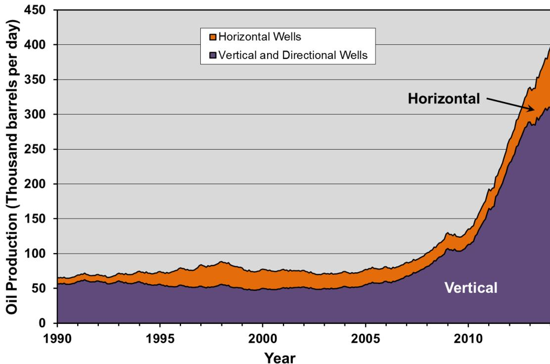
**Figure 2-59. Oil production from the Spraberry play by well type.<sup>94</sup>**
