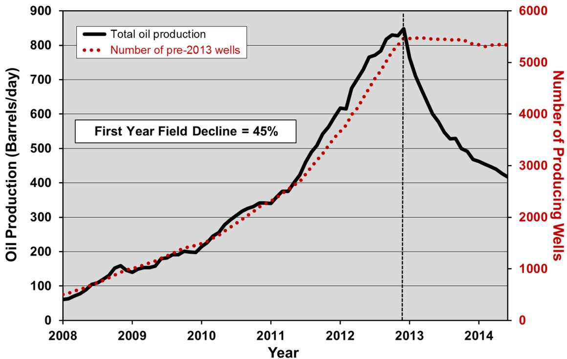
**Figure 2-14. Production rate and number of horizontal tight oil wells in the Bakken play prior to 2013.<sup>27</sup>**
