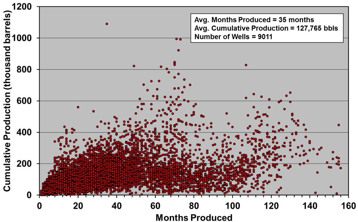
**Figure 2-16. Cumulative oil production and length of time produced for Bakken wells that were producing as of March 2014.<sup>29</sup>**
