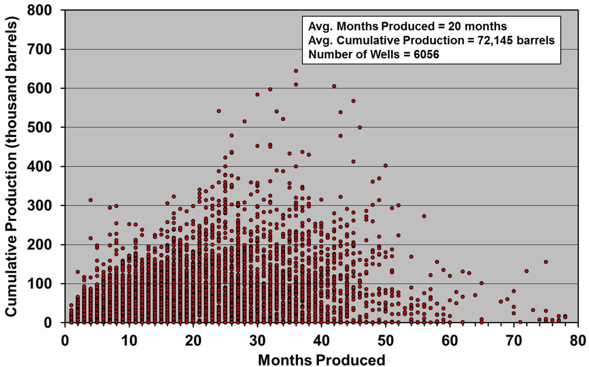
**Figure 2-37. Cumulative oil production and months produced for Eagle Ford wells that were producing as of March 2014.<sup>64</sup>**
