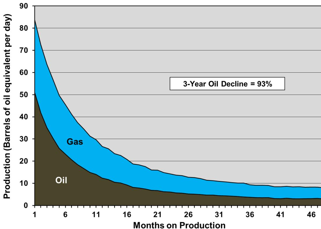
**Figure 2-88. Oil and gas average well decline profile for all wells in the Niobrara-Codell play.**<sup>135</sup>
