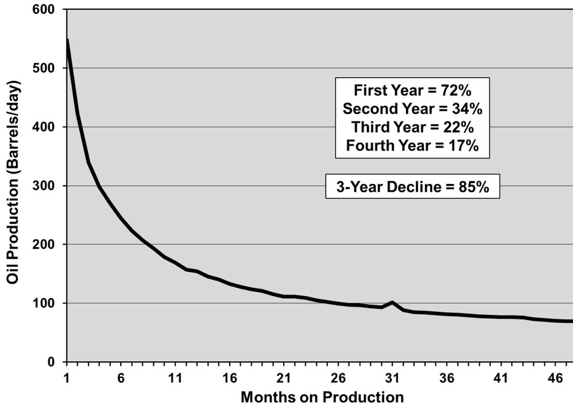
**Figure 2-13. Average decline profile for horizontal tight oil wells in the Bakken play.<sup>25</sup>**
