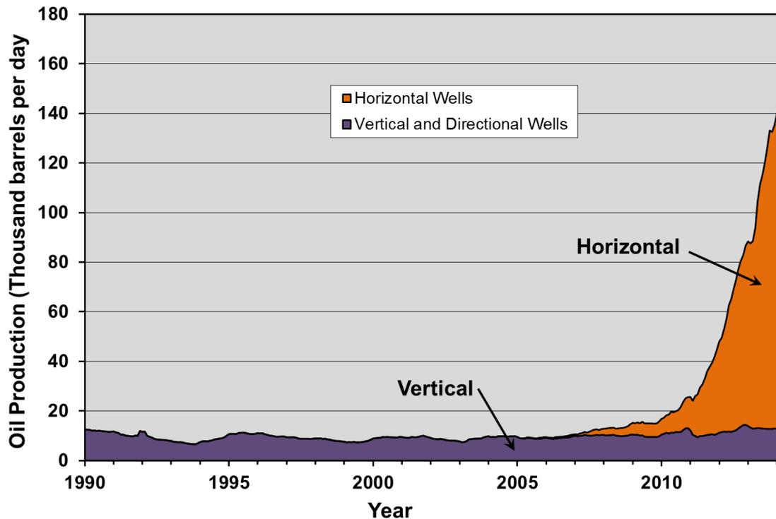
**Figure 2-71. Oil production from the Bone Spring play by well type.<sup>108</sup>**
