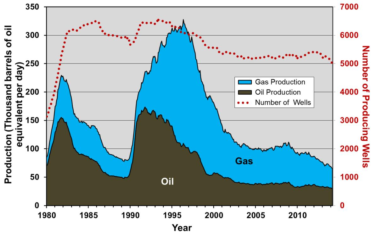
**Figure 2-79. Austin Chalk play oil and gas production and number of producing wells, 1980 to 2014.**<sup>125</sup>
