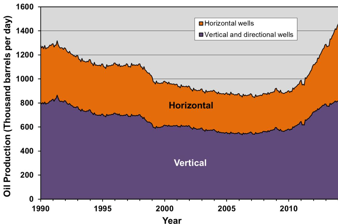
**Figure 2-56. Oil production by well type in the Permian Basin, 1990 to 2014.<sup>91</sup>**
