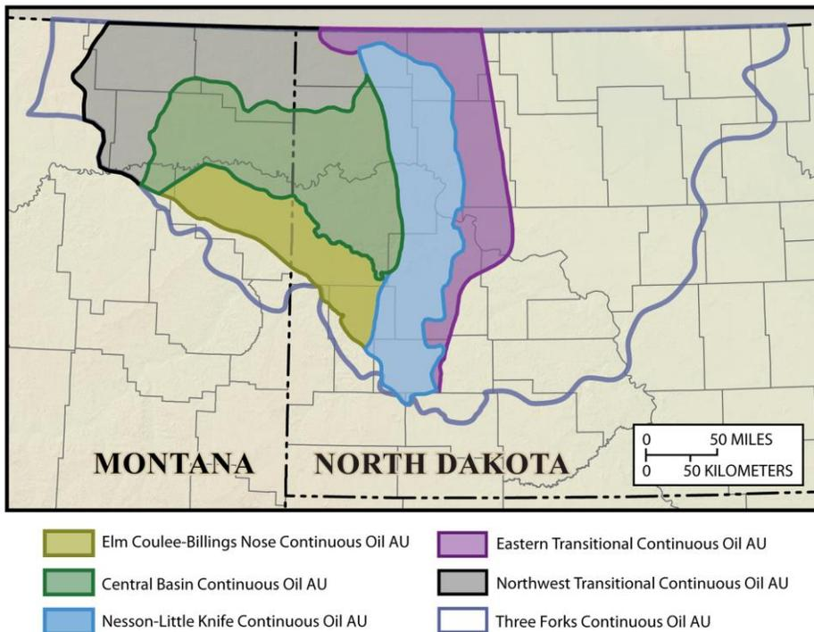
**Figure 2-8. USGS demarcation of Bakken and Three Forks tight oil assessment units.<sup>16</sup>**
