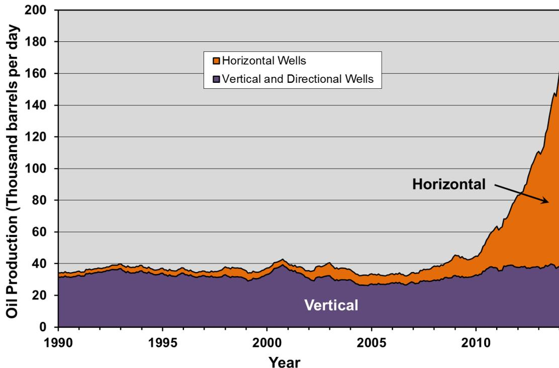
**Figure 2-65. Oil production from the Wolfcamp play by well type.<sup>101</sup>**
