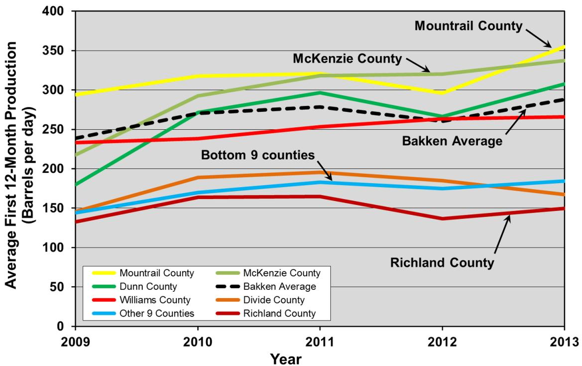
**Figure 2-23. Average first-year oil production rates of wells in the Bakken play by county, 2009 to 2013.<sup>38</sup>**
