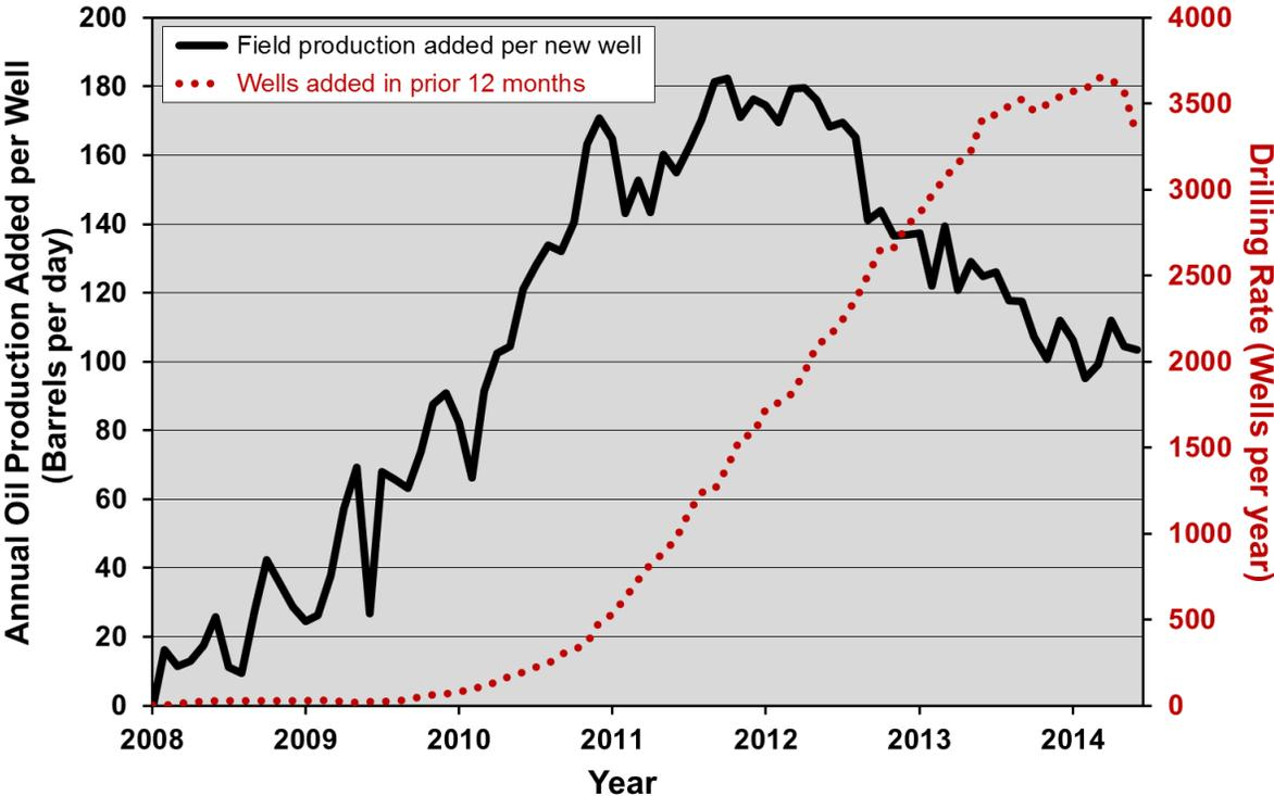
Figure 2-32. Annual oil production added per new well and annual drilling rate in the Eagle Ford play, 2008 through 2014, 2008 to 2014.<sup>59</sup>
