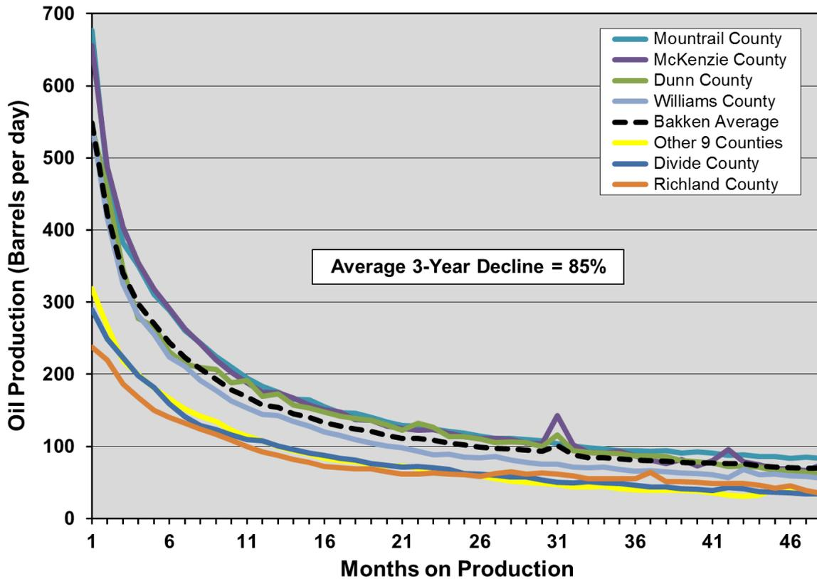
**Figure 2-21. Average tight oil well decline profiles by county for the Bakken play.<sup>35</sup>**
