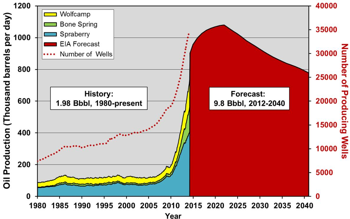
**Figure 2-76. Oil production and number of producing wells in the Spraberry, Wolfcamp, and Bone Spring plays to 2014, with EIA reference case projection for these plays through 2040.<sup>115</sup>**
