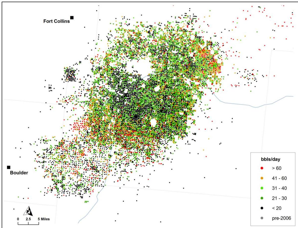
**Figure 2-85. Detail of Niobrara-Codell play showing distribution of wells as of mid-2014, illustrating highest one-month oil production (initial productivity, IP).<sup>132</sup>**
