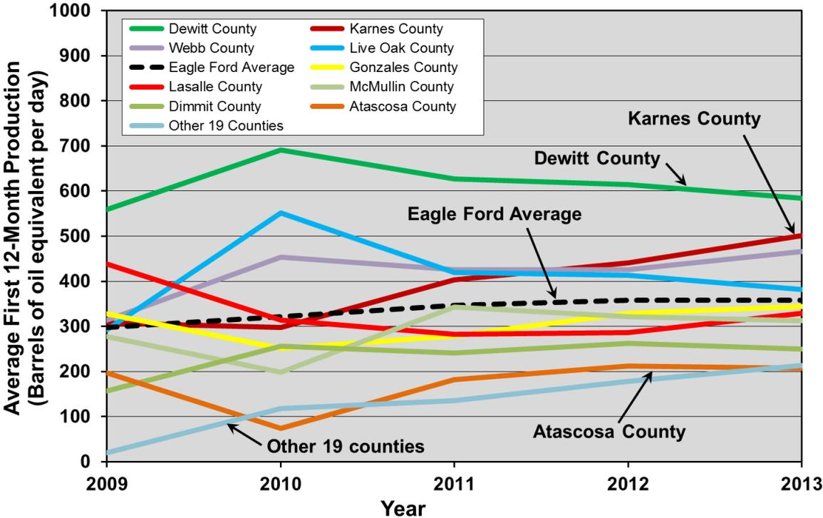
**Figure 2-49. Average first-year oil and gas production rates of wells on a “barrels of oil equivalent” basis by county for the Eagle Ford play, 2009 to 2013.<sup>78</sup>**
