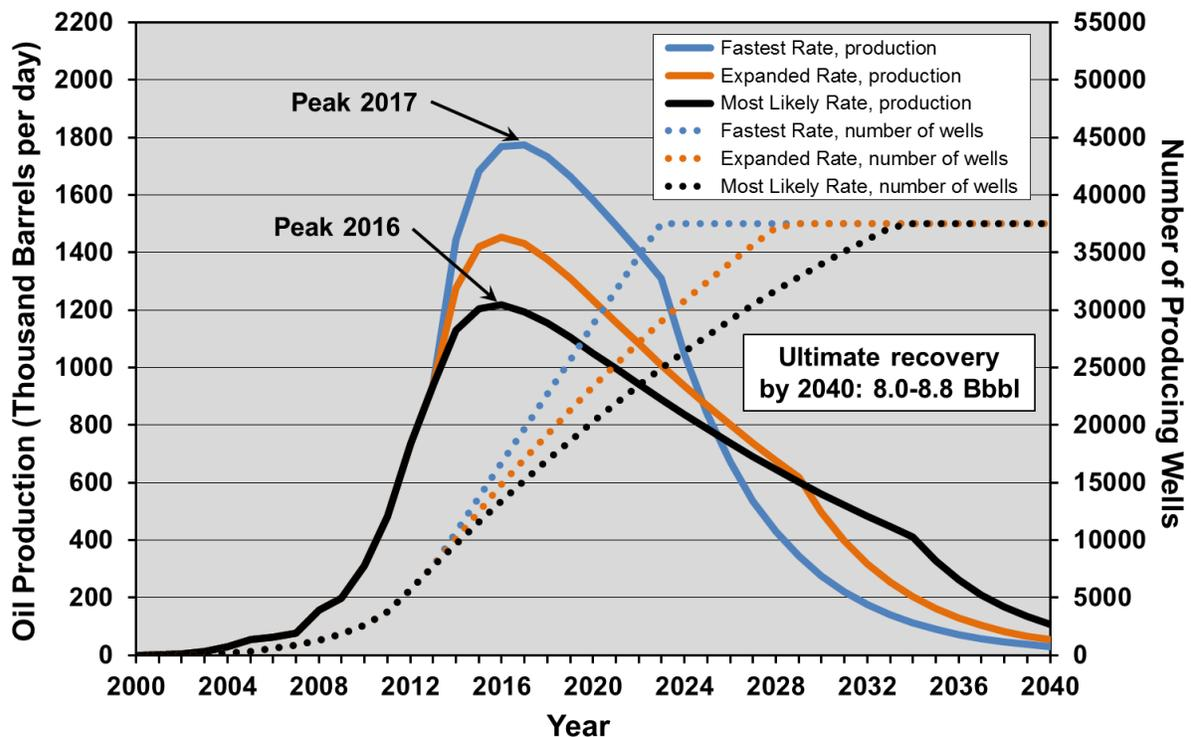
**Figure 2-25. Three drilling rate scenarios of Bakken tight oil production, in the “Optimistic Case” (100% of play area is drillable at three wells per square mile).<sup>47</sup>**
