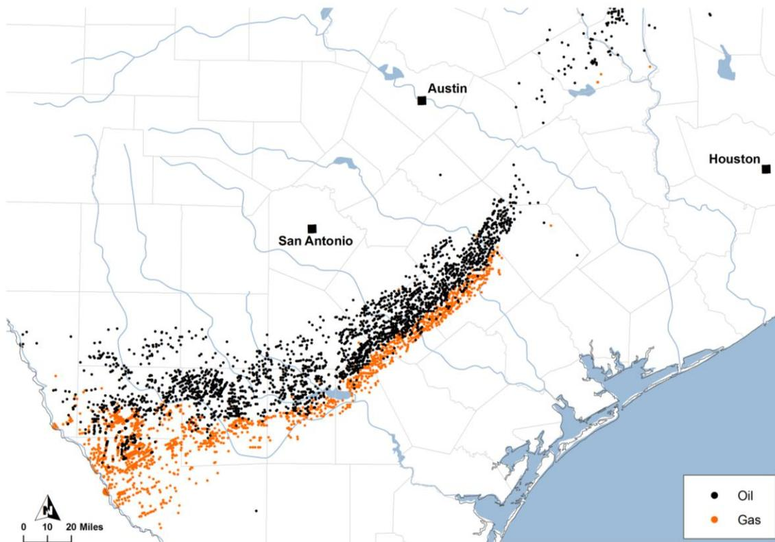
**Figure 2-30. Distribution of oil and gas wells in the main portion of the Eagle Ford play as of early 2014.<sup>57</sup>**
