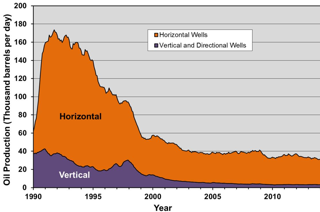
**Figure 2-80. Oil production from the Austin Chalk play by well type.<sup>126</sup>**
