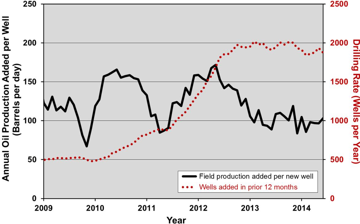
Figure 2-12. Annual oil production added per new well and annual drilling rate in the Bakken play, 2009 through 2014.<sup>24</sup>
