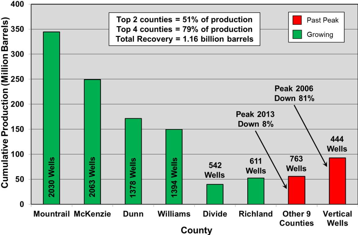
**Figure 2-19. Cumulative oil production by county in the Bakken play through 2014.<sup>32</sup>**
