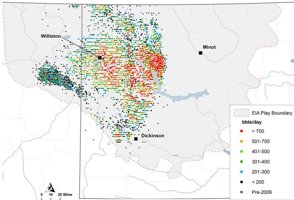
**Figure 2-9. Distribution of wells in the Bakken play as of mid-2014 illustrating highest one-month oil production (initial productivity, IP),<sup>17</sup> with EIA play boundary.<sup>18</sup>**
