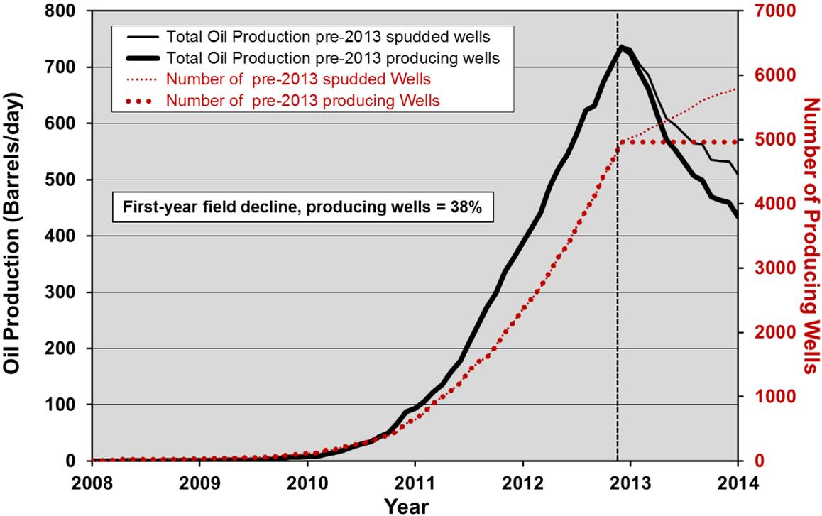
**Figure 2-34. Production rate and number of horizontal tight oil wells in the Eagle Ford spudded or producing prior to 2013.<sup>61</sup>**
