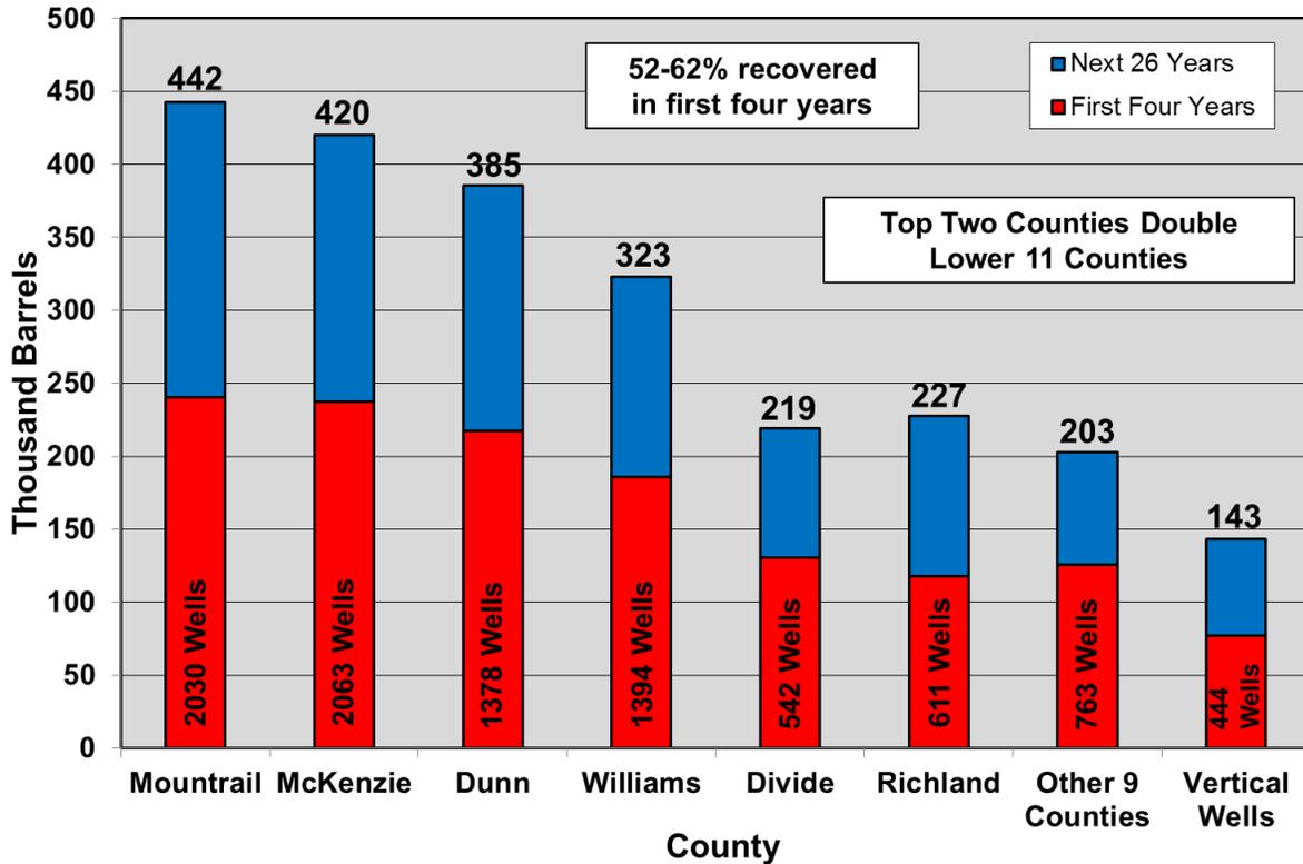
**Figure 2-22. Estimated ultimate recovery of oil per well by county for the Bakken play.<sup>37</sup>**
