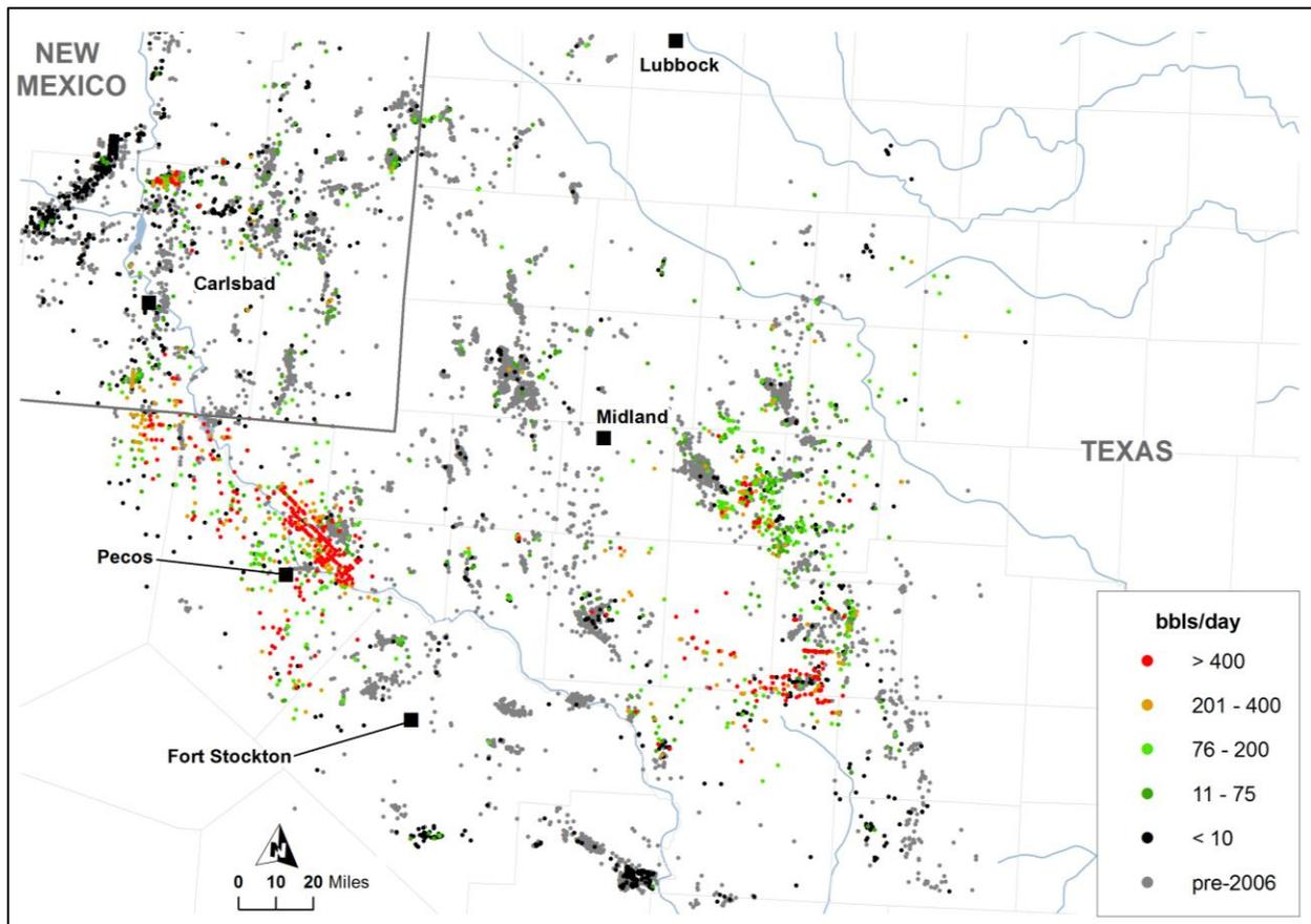
**Figure 2-63. Distribution of wells in the Wolfcamp play as of mid-2014 illustrating highest one-month oil production (initial productivity, IP).<sup>99</sup>**
