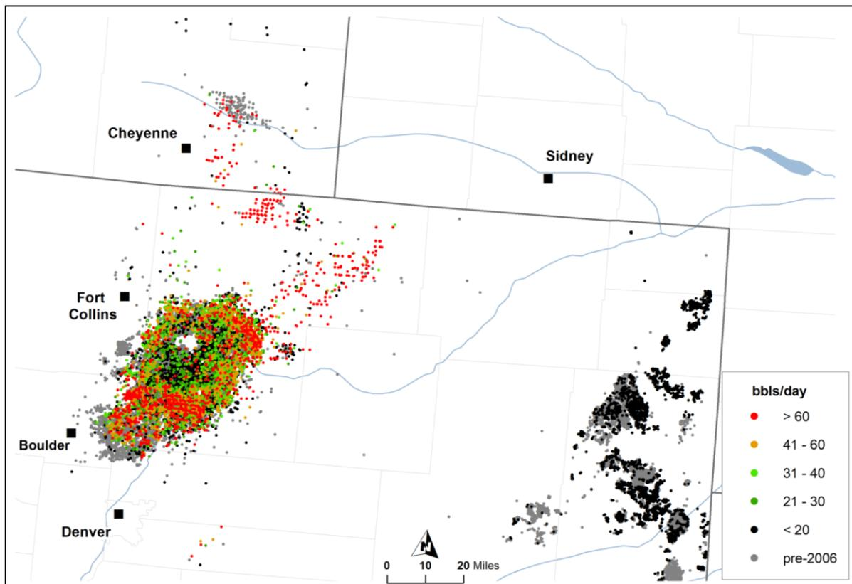
**Figure 2-84. Distribution of wells in the Niobrara-Codell play as of mid-2014 illustrating highest one-month oil production (initial productivity, IP).<sup>131</sup>**
