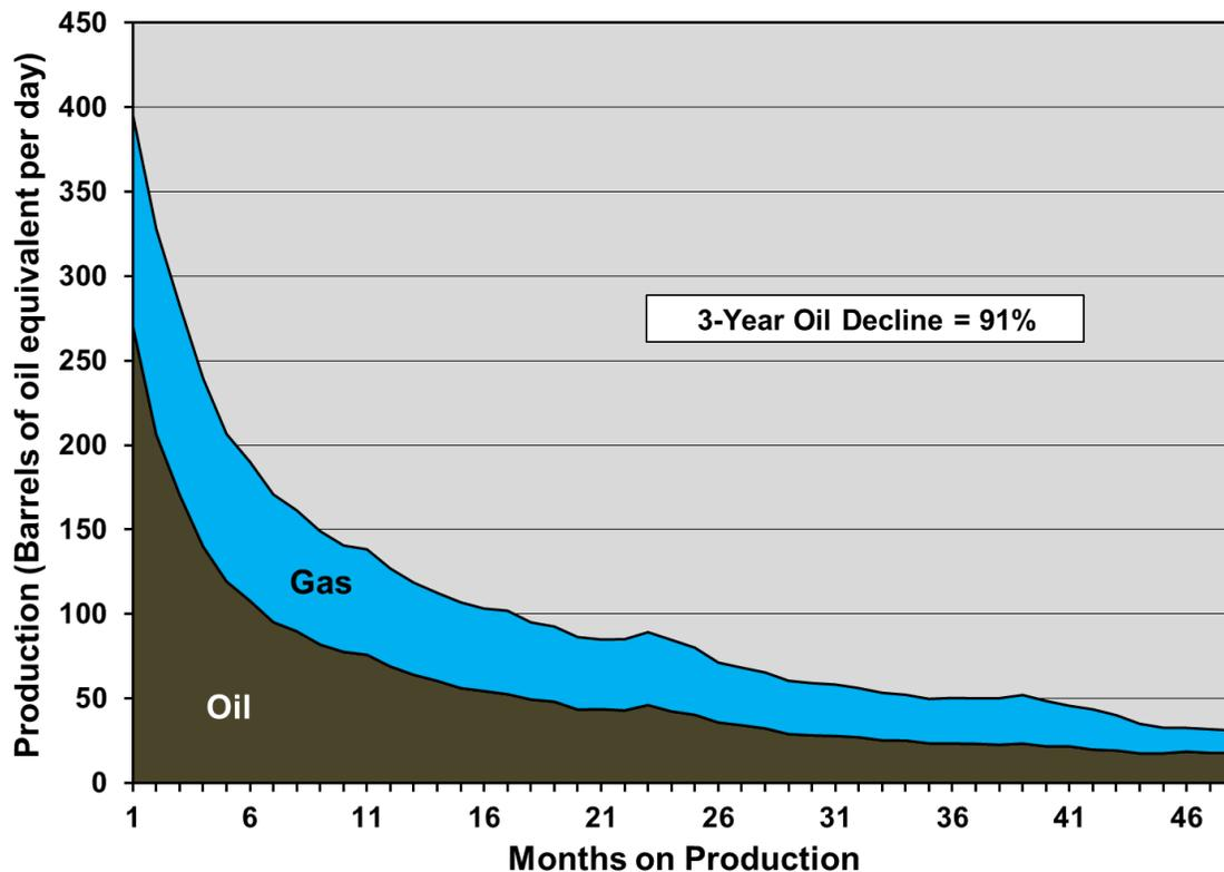
**Figure 2-72. Oil and gas average well decline profile for all wells in the Bone Spring play.<sup>109</sup>**
