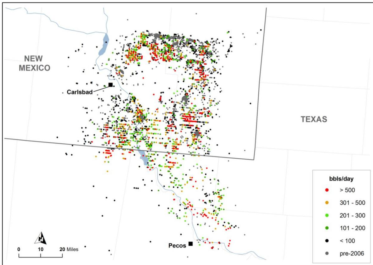
**Figure 2-69. Distribution of wells in the Bone Spring play as of mid-2014 illustrating highest one-month oil production (initial productivity, IP).<sup>106</sup>**
