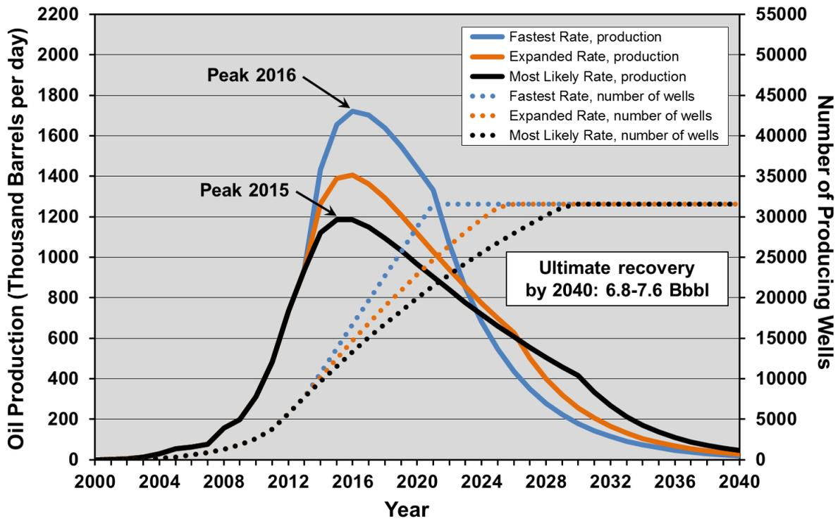
**Figure 2-26. Three drilling rate scenarios of Bakken tight oil production, in the “Realistic Case” (80% of the remaining play area is drillable at three wells per square mile).<sup>48</sup>**
