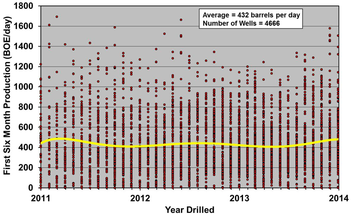
**Figure 2-39. Average oil and gas production over the first six months for all wells drilled in the Eagle Ford play on a barrels of oil equivalent basis.<sup>66</sup>**
