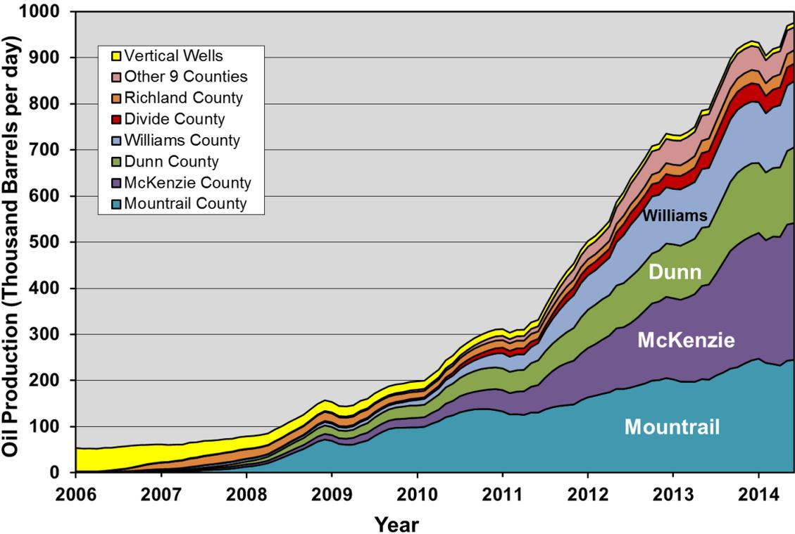
**Figure 2-18. Oil production by county in the Bakken play, 2006 through 2014.<sup>31</sup>**
