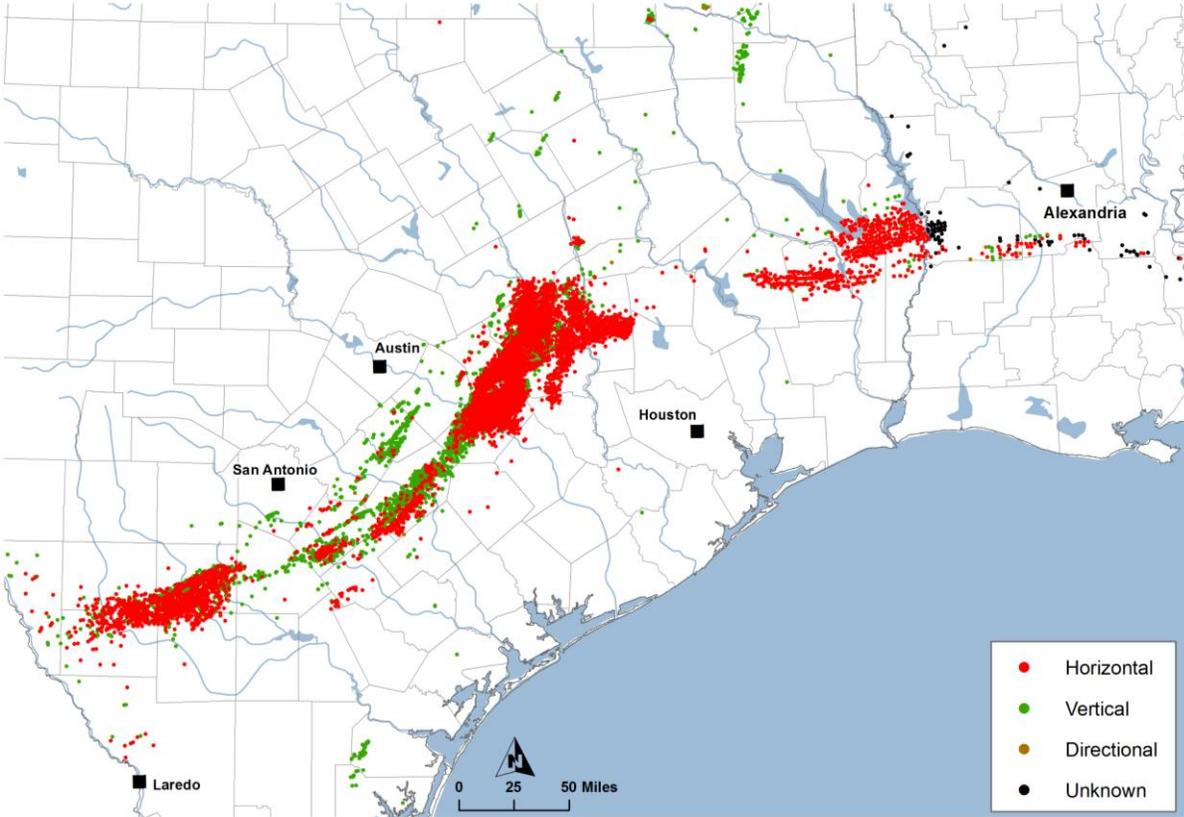
**Figure 2-78. Distribution of wells in the Austin Chalk play categorized by drilling type, as of early 2014.<sup>124</sup>**
