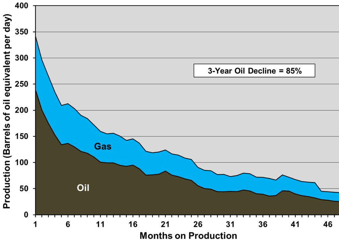
**Figure 2-67. Oil and gas average well decline profile for horizontal wells in the Wolfcamp play.<sup>103</sup>**
