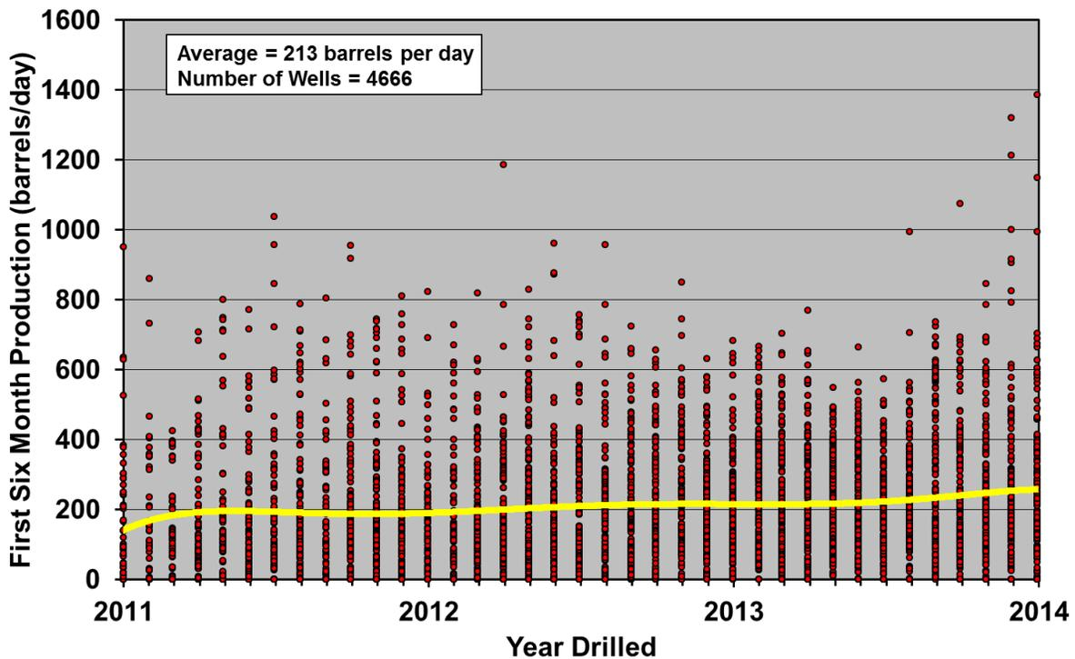
**Figure 2-38. Average oil production over the first six months for all wells drilled in the Eagle Ford play.<sup>65</sup>**
