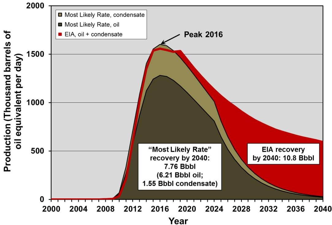
**Figure 2-53. "Most Likely Rate" scenario ("Realistic" case) of Eagle Ford tight oil production compared to the EIA reference case, 2000 to 2040.<sup>86</sup>**
