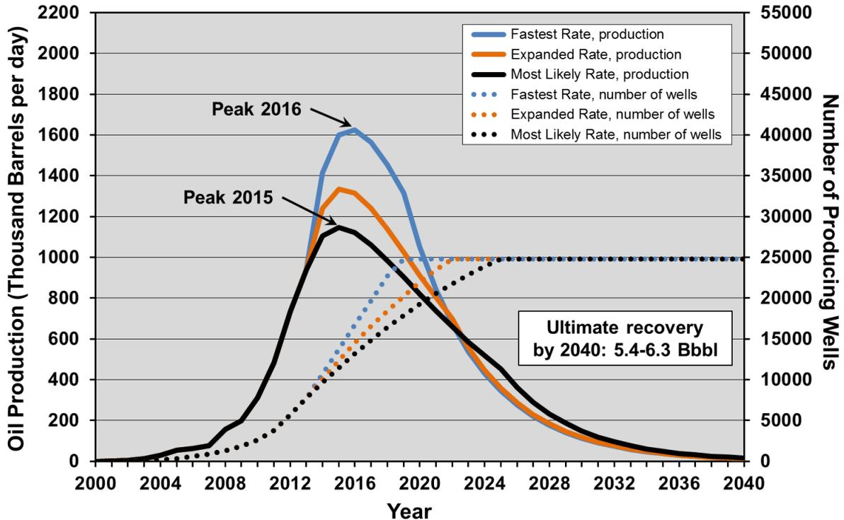
**Figure 2-24. Three drilling rate scenarios of Bakken tight oil production, in the “Low Well Density Case” (100% of play area is drillable at two wells per square mile).<sup>46</sup>**
