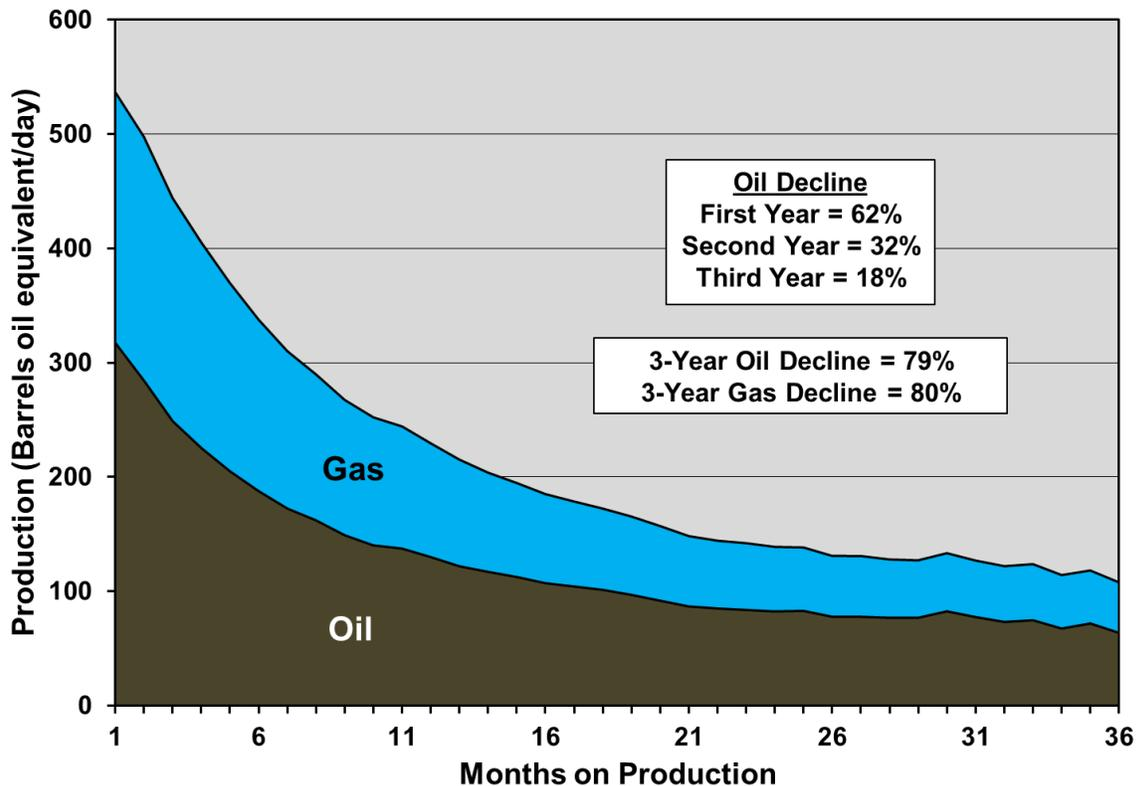
**Figure 2-33. Average decline profile for horizontal tight oil and shale gas wells in the Eagle Ford play.<sup>60</sup>**
