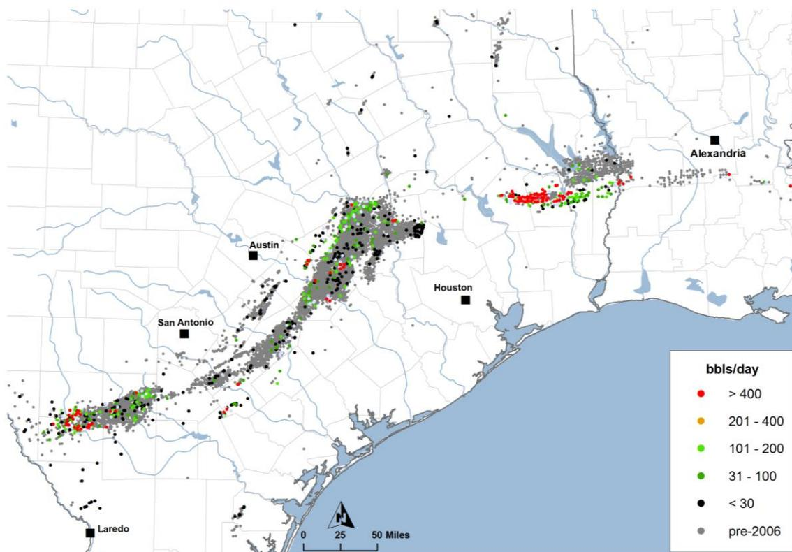
**Figure 2-77. Distribution of wells in the Austin Chalk play as of mid-2014 illustrating highest one-month oil production (initial productivity, IP).<sup>123</sup>**
