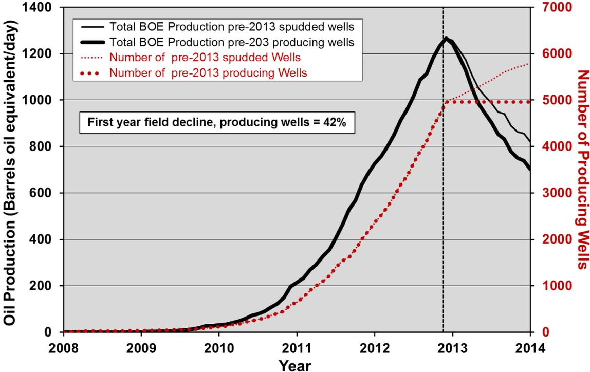
**Figure 2-35. Production rate and number of horizontal tight oil wells in the Eagle Ford spudded or producing prior to 2013, including gas on a “barrels of oil equivalent” basis.<sup>62</sup>**
