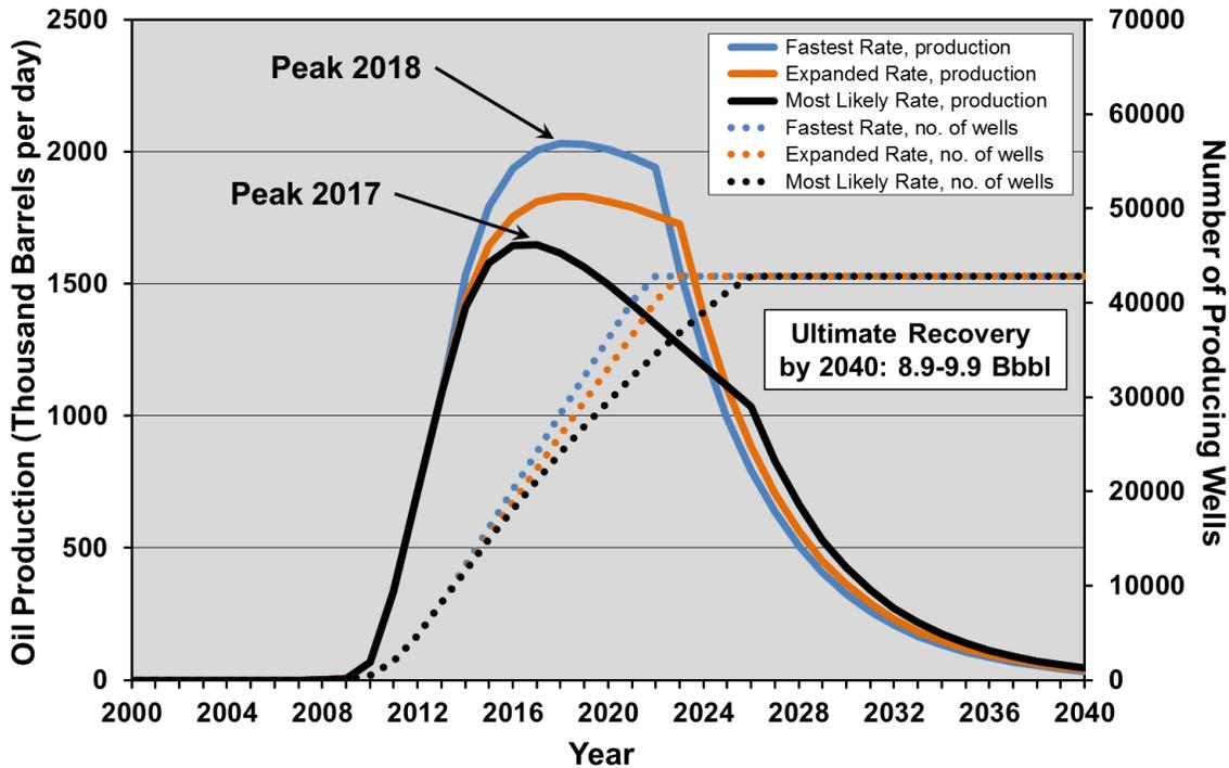
**Figure 2-50. Three drilling rate scenarios of Eagle Ford tight oil production, in the “Optimistic Case” (100% of the play area is drillable at six wells per square mile).<sup>82</sup>**
