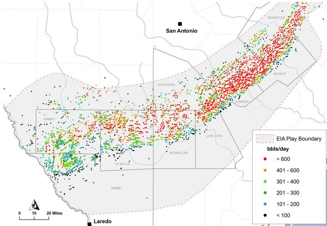
**Figure 2-29. Detail of Eagle Ford play showing distribution of wells as of mid-2014 illustrating highest one-month oil production (initial productivity, IP),<sup>55</sup> with EIA play boundary.<sup>56</sup>**
