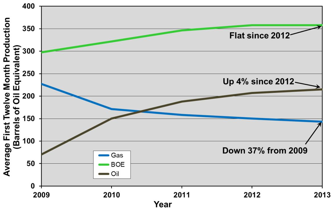
**Figure 2-36. Average first year production rates for Eagle Ford wells from 2009 to 2013.**<sup>63</sup>
