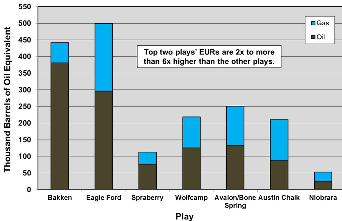
**Figure 2-93. Estimated ultimate recovery (EUR) of oil and gas per well of reviewed plays, on a “barrels of oil equivalent” basis.<sup>154</sup>**
