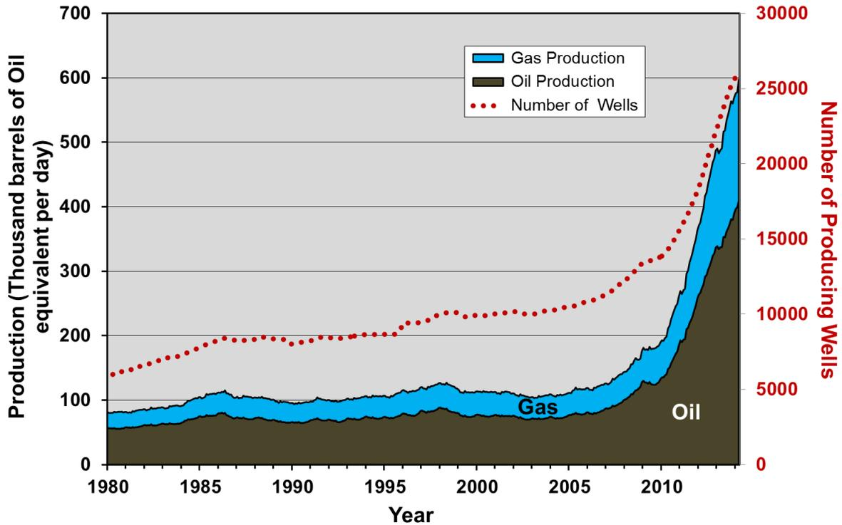
**Figure 2-58. Spraberry play oil and gas production and number of producing wells, 1980 to 2014.<sup>93</sup>**
