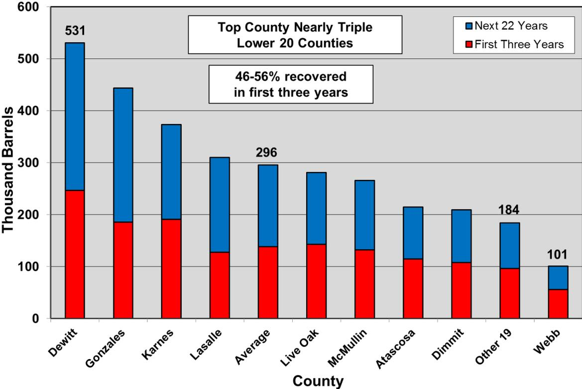
**Figure 2-46. Estimated ultimate recovery of oil per horizontal well by county for the Eagle Ford play.<sup>75</sup>**
