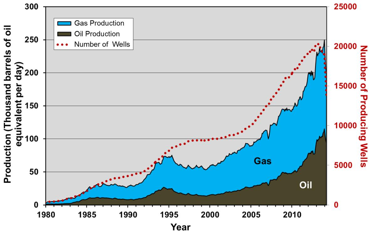
**Figure 2-86. Niobrara-Codell play oil and gas production and number of producing wells, 1980 to 2014.**<sup>133</sup>
