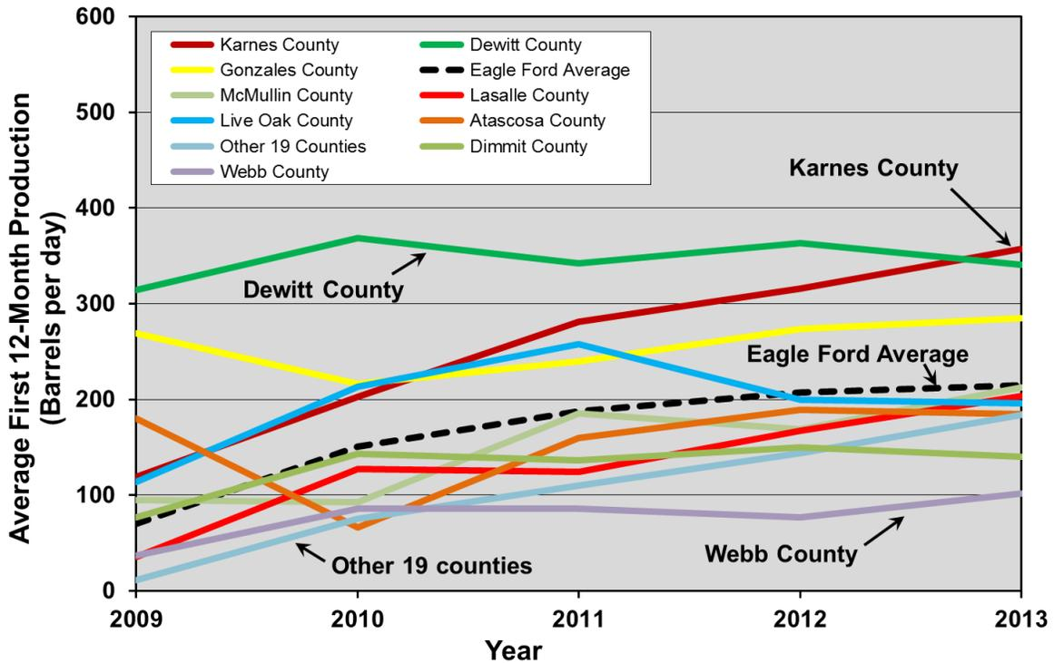
**Figure 2-48. Average first-year oil production rates of wells by county for the Eagle Ford play, 2009 to 2013.<sup>77</sup>**
