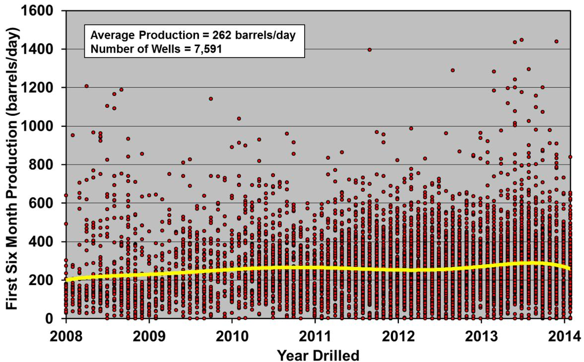
**Figure 2-17. Average oil production over the first six months for all wells drilled in the Bakken play, 2008-2014.<sup>30</sup>**
