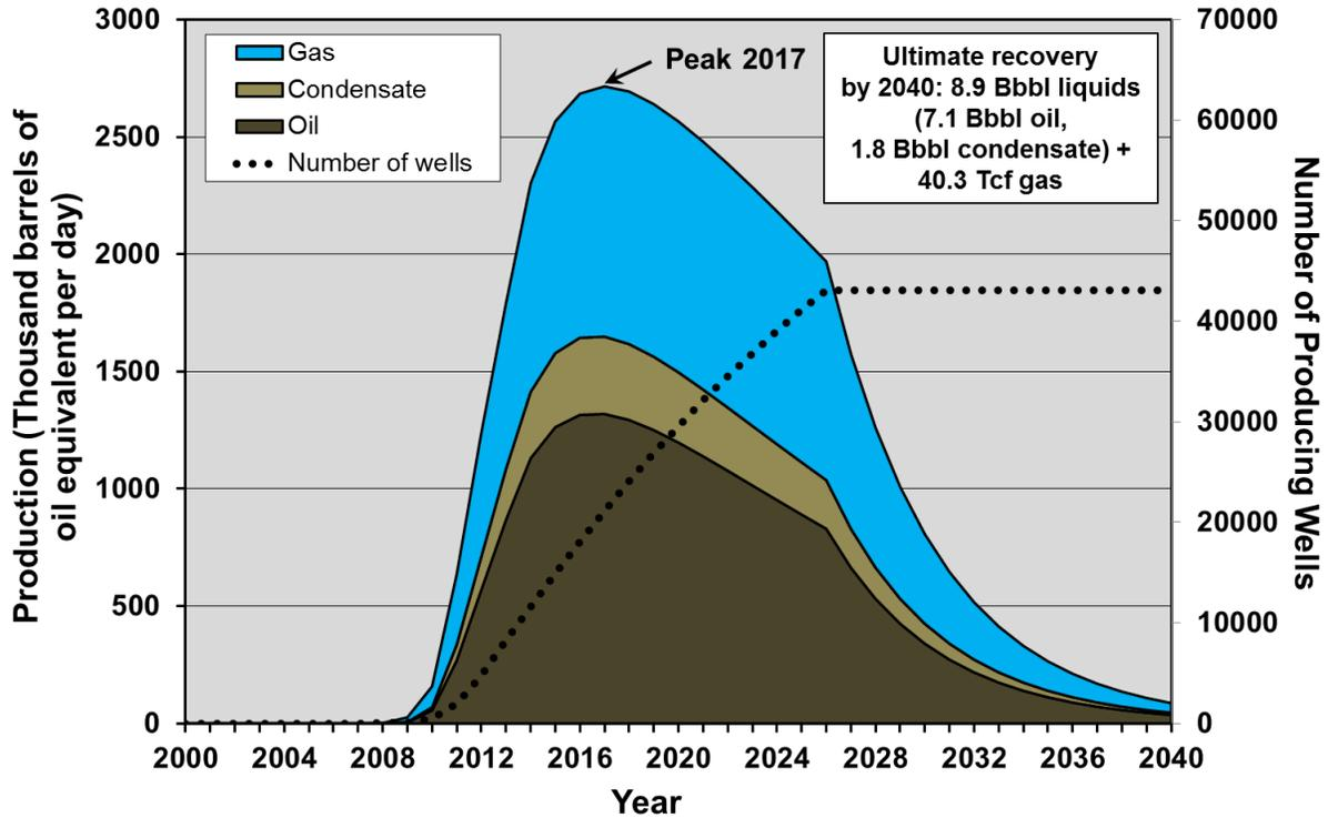
**Figure 2-51. “Most Likely Rate” scenario of Eagle Ford production for oil, condensate and gas in the “Optimistic” case (100% of the play area is drillable at six wells per square mile).<sup>84</sup>**
