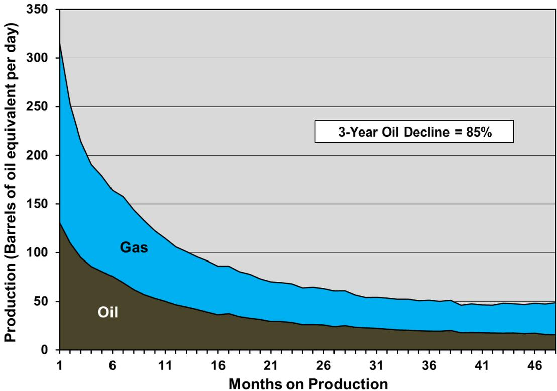
**Figure 2-82. Oil and gas average well decline profile for horizontal wells in the Austin Chalk play.<sup>128</sup>**
