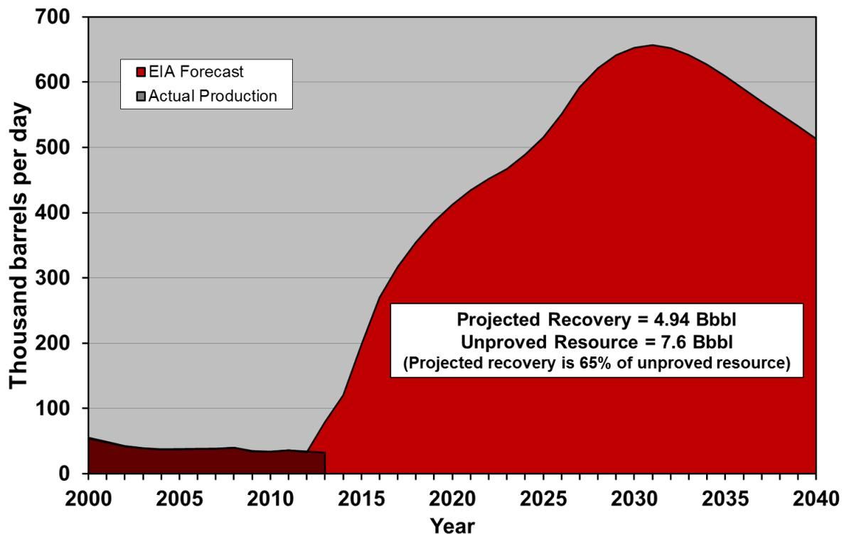
**Figure 2-83. EIA reference case projection of oil production from the Austin Chalk through 2040, with actual production to 2013.<sup>129</sup>**
