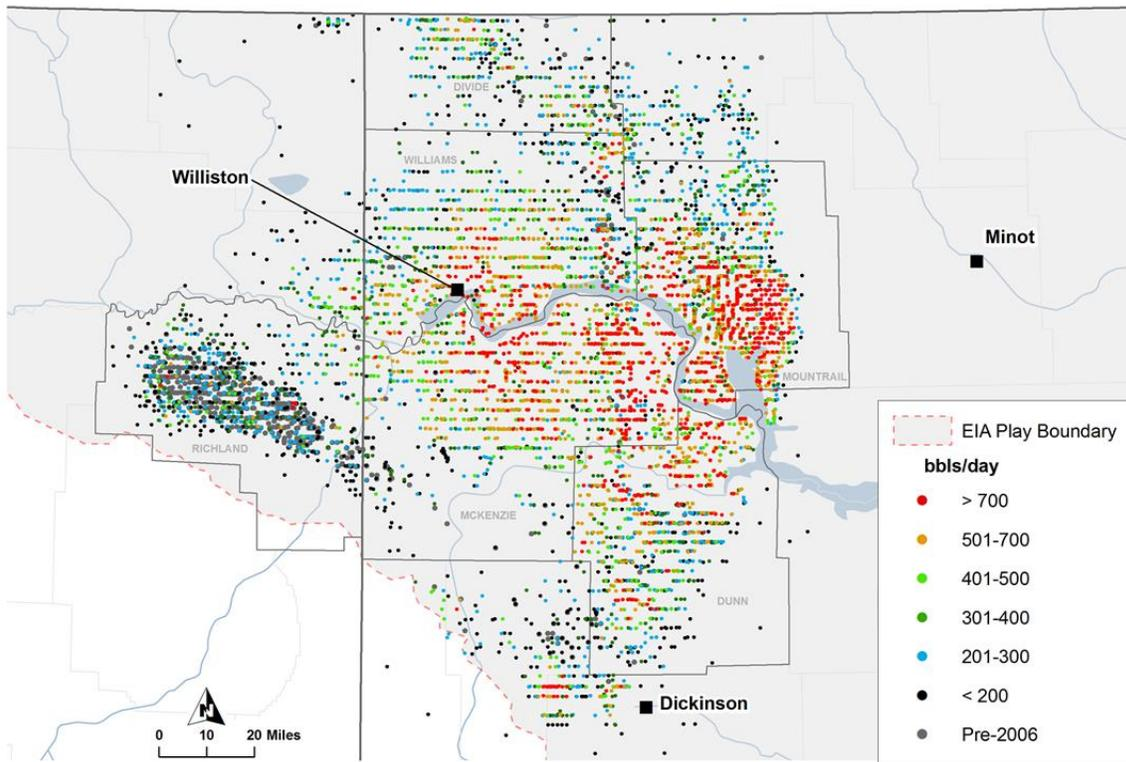
**Figure 2-10. Detail of Bakken play showing distribution of wells as of early 2014, and illustrating highest one-month oil production (initial productivity, IP),<sup>20</sup> with EIA play boundary.<sup>21</sup>**
