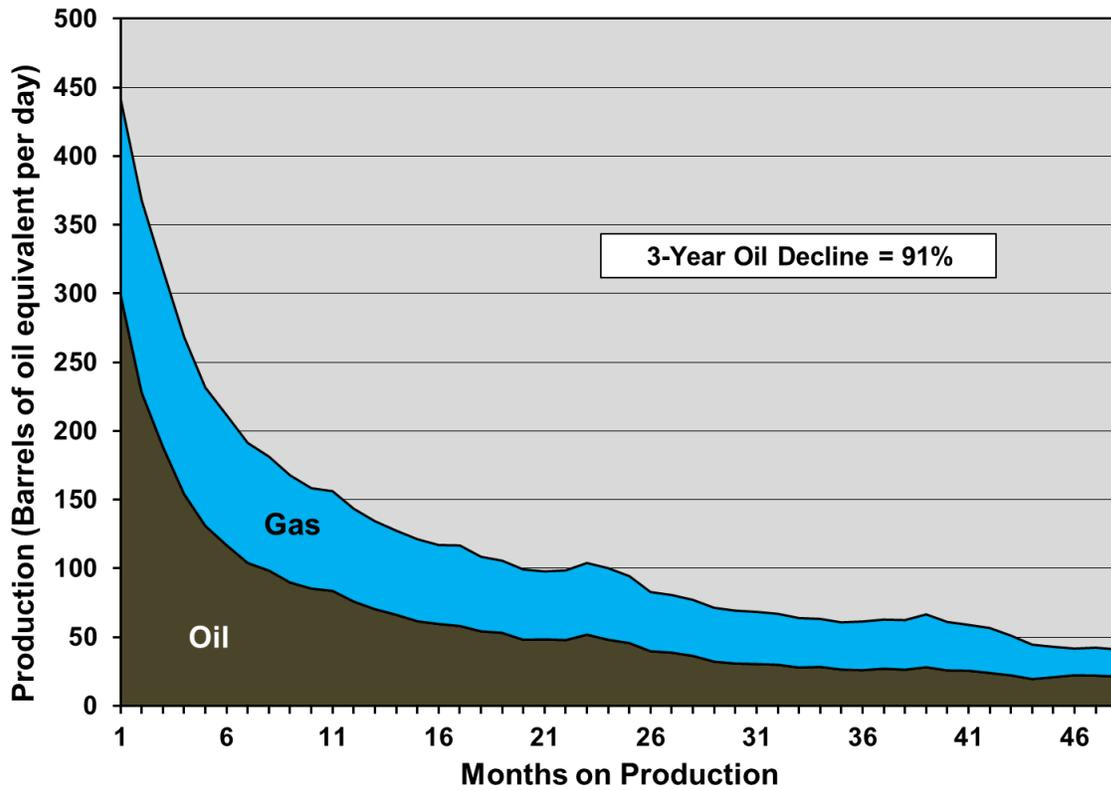
**Figure 2-73. Oil and gas average well decline profile for horizontal wells in the Bone Spring play.<sup>110</sup>**
