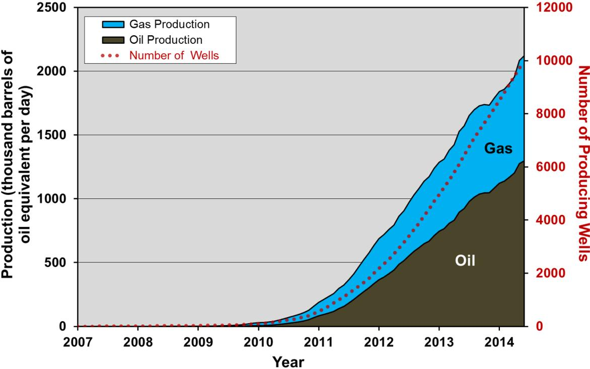
**Figure 2-31. Eagle Ford play tight oil and gas production and number of producing wells, 2007 to 2014.<sup>58</sup>**
