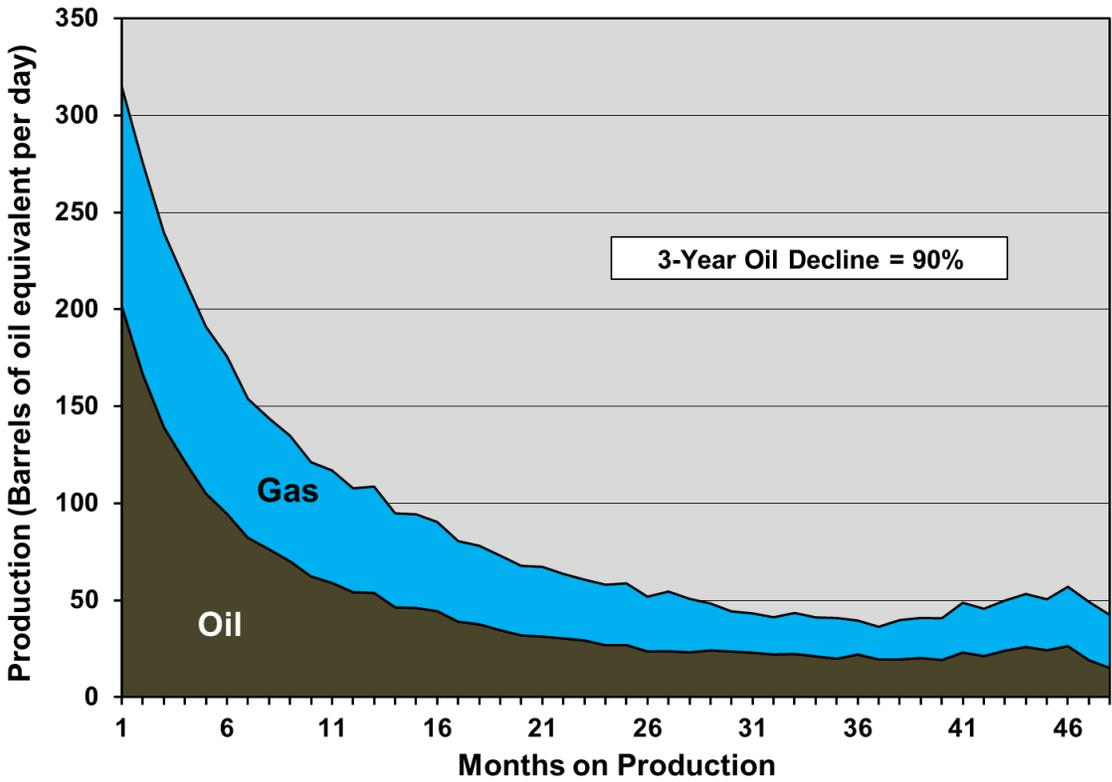
**Figure 2-89. Oil and gas average well decline profile for horizontal wells in the Niobrara-Codell play.<sup>136</sup>**
