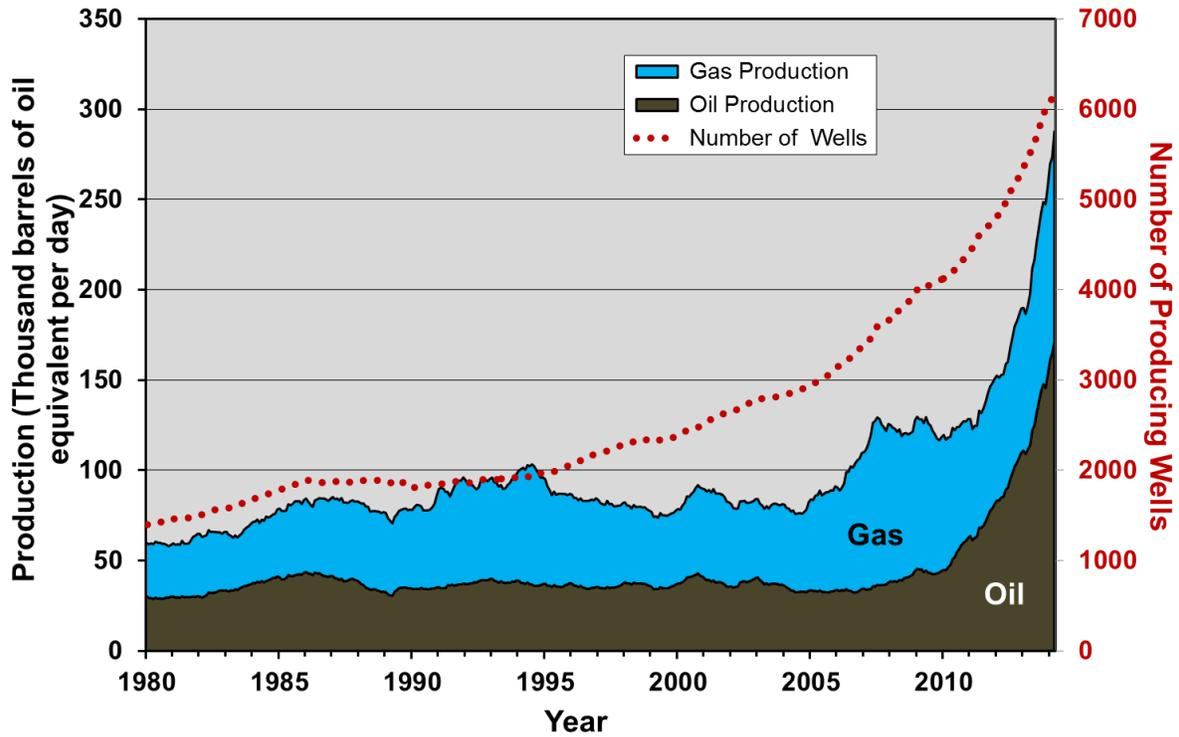
**Figure 2-64. Wolfcamp play oil and gas production and number of producing wells, 1980 to 2014.<sup>100</sup>**
