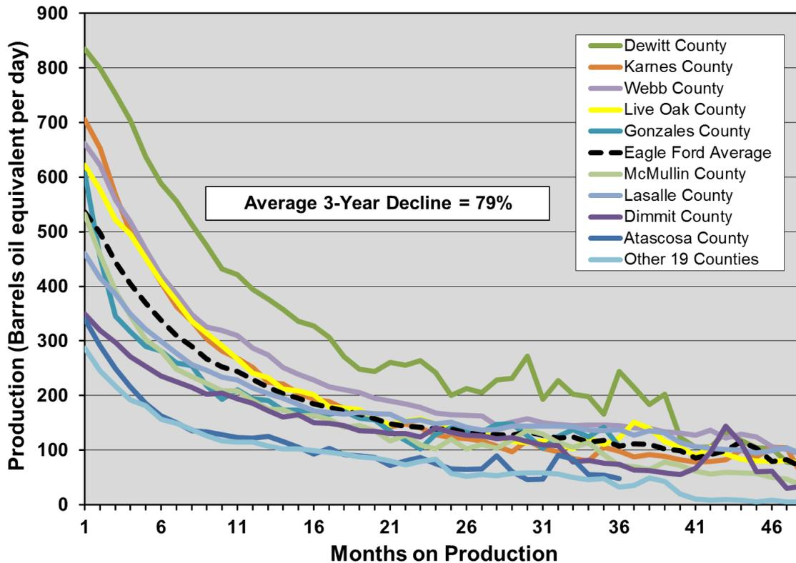
**Figure 2-45. Average well decline profiles on a “barrels of oil equivalent” basis including the energy of natural gas produced by county for the Eagle Ford play.<sup>73</sup>**
