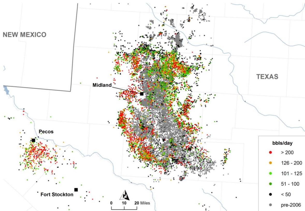
**Figure 2-57. Distribution of wells in the Spraberry play as of mid-2014 illustrating highest one-month oil production (initial productivity, IP).<sup>92</sup>**
