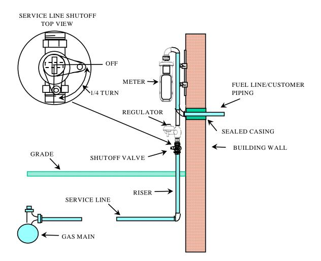
Note that the shutoff valve is before the regulator and meter. This valve must be designed so that it can be locked in the closed position. Depending on the type of valve, more than a quarter turn may be required to shut off gas.
