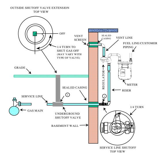
The service can be shut off at either point (1) or (2). Note that the shutoff valve at point (1) is installed before the regulator. The valve at point (1) must be designed so that it can be locked in a closed position. Depending on the type of valve, more than a quarter turn may be required to shut off gas.
