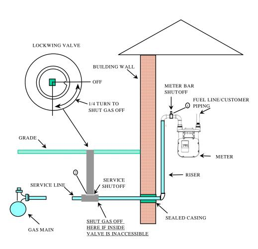
Note that this service can be shut-off at either points (1) or (2). The valve at point (1) must be designed so that it can be locked in a closed position. The valve at point (2) is installed in a valve box. Depending on the type of valve, more than a quarter turn may be required to shut-off gas.
