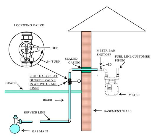
This is a typical low-pressure service (pressure in main and service are essentially the same as customer utilization pressure). Note that this service can be shut off at either (1) or (2) as shown on drawing. This service would be in compliance with 49 CFR 192.365. The valve at either points (1) or (2) must be designed so that it can be locked in a closed position. Depending on the type of valve, more than a quarter turn may be required to shut off gas.
