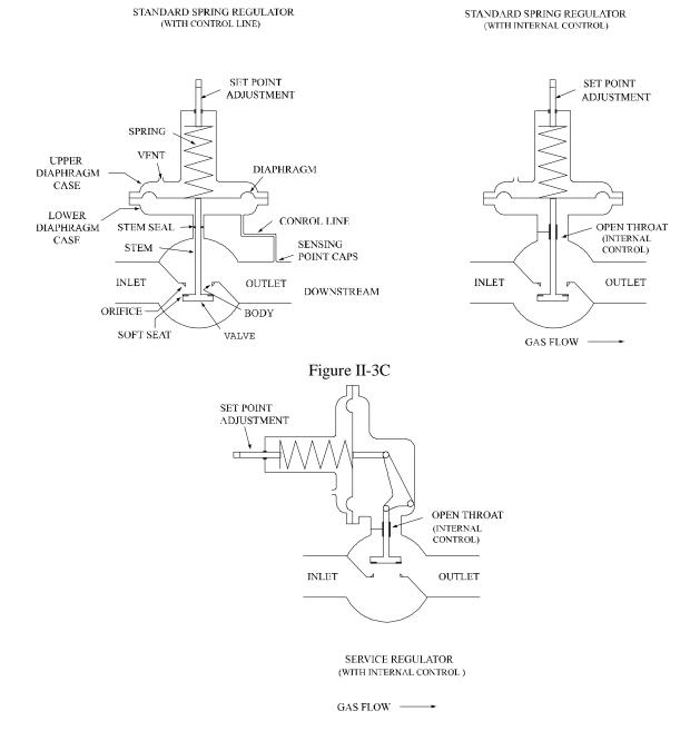
FIGURE II-3 shows a simple section of a standard spring regulator. The various parts are labeled. For most master meter operators this will be the only type of regulator in the system. Service regulators are this type of regulator. Referring to FIGURE II-3, the following is a simple explanation of how it works.
