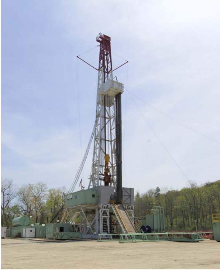
Photo 5.14 Triple. Precision Drilling Rig 26. Ruger 1 well, Horseheads, Chemung County. Credit: NYS DEC 2009.
