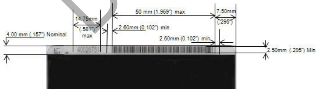
Figure 1 – Barcode and Serial Number Placement and Dimensions
