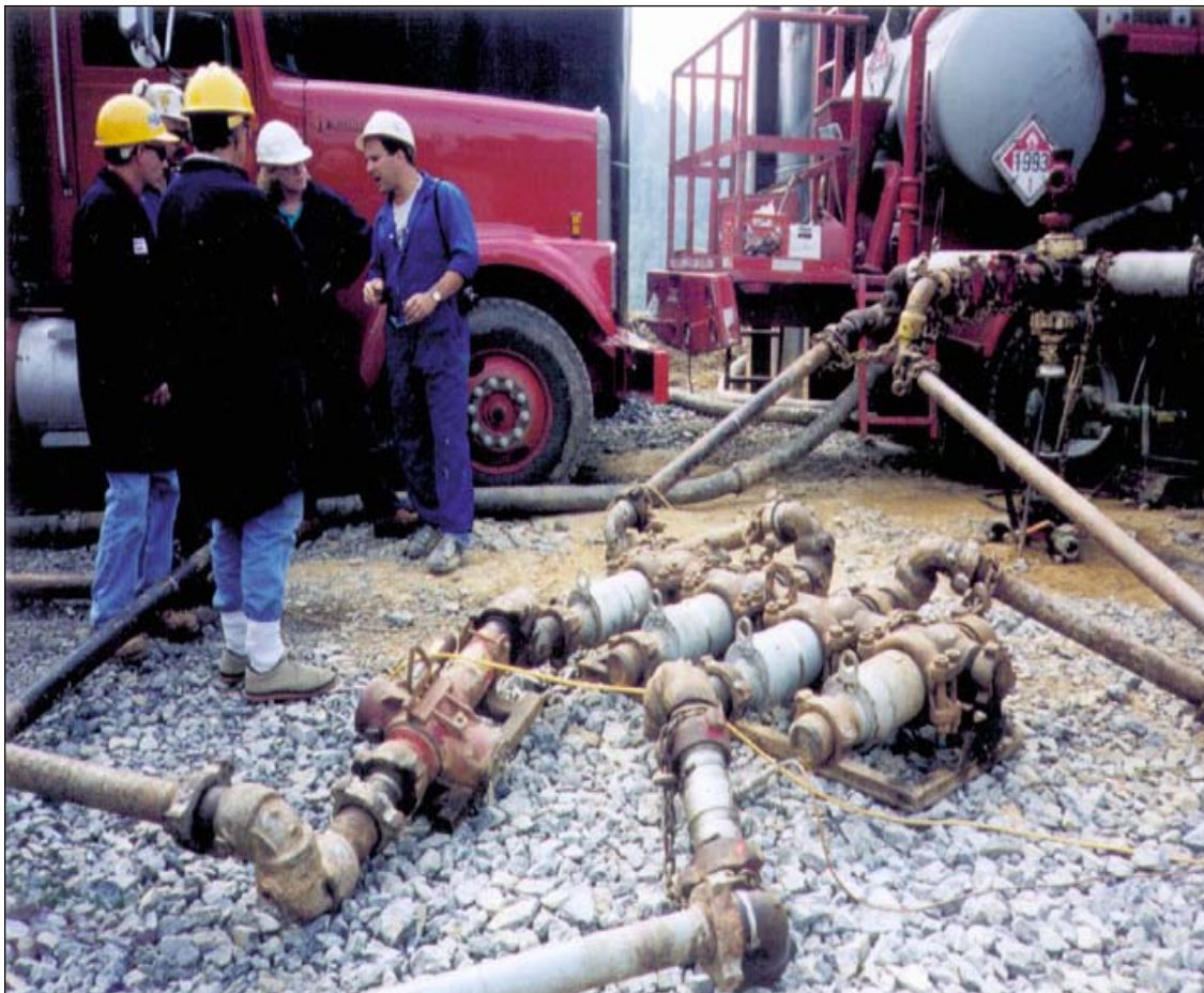
Figure 4-7. The fracturing fluids, additives, and proppant are pumped to the wellhead and mixed just prior to injection. The flow rate of each injected component is monitored carefully from an on-site control center.
